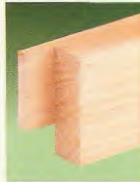
▲ Tongue Detail. Tongues cut on the ends of the hanger strip fit into the rabbets in the sides of the storage rack.
