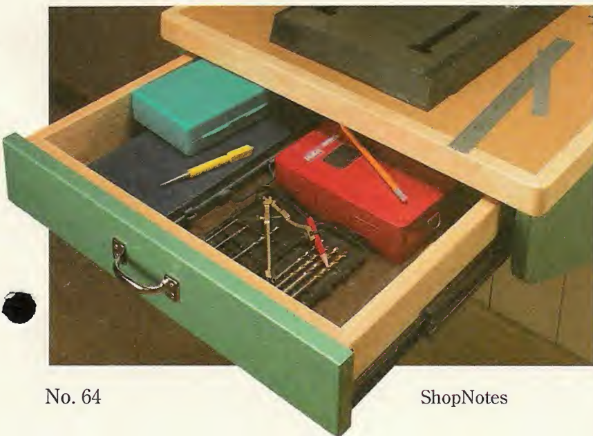
◀ Drawer. The drawer rides on full-extension drawer slides, making it easy to reach items at the back.
