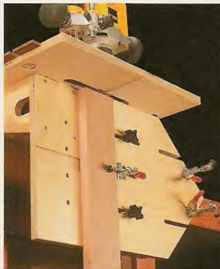
▲ Vertical Workpieces. To rout a mortise on the end of a workpiece, simply rotate the sliding plate 90° to the base.
