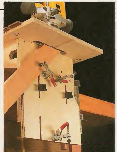
▲ Mitered Workpieces. For mortising mitered workpieces, the sliding plate can be turned upside down.
