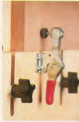
▲ Adjustable. Slots in the sliding plate allow you to adjust the jig for different size workpieces. And a toggle clamp holds the workpiece securely in place.
