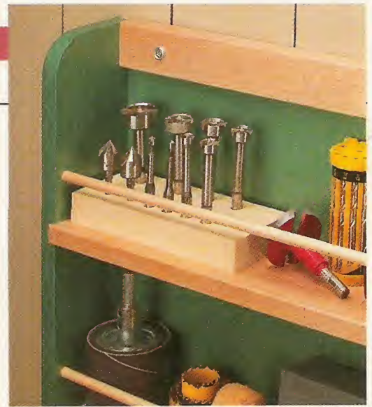
▲ Guard Rail. Like the guard rail on a highway, the shelf rails on this storage rack prevent items from falling off the edges of the shelves.
