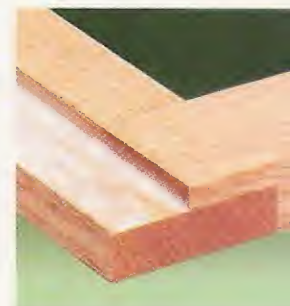
▲ Cleaner Glue-ups. You'll have less glue squeeze out on the inside of the cabinet if you only spread the glue to the corner of the rabbet.
