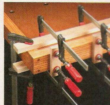
▲ "Stretching" Your Clamps. A couple of cleats attached to the top of the bench allow you to clamp the end apron in place.
