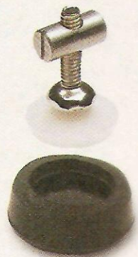
▲ Clamp Pad. To make the clamp pad, thread a leg leveler into a barrel nut. Then cut off the end of a rubber crutch tip and slip it over the leg leveler.
