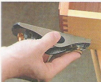
▲ Low-Angle Block Plane. A low-angle block plane is a good choice for cutting end grain, like the pins on this dovetail joint.
