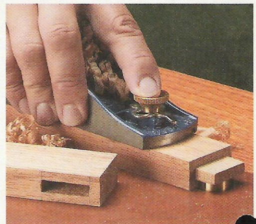
▲ Block Plane. A block plane can quickly trim a rail so it's flush with a stile, either before or after the pieces are assembled.
