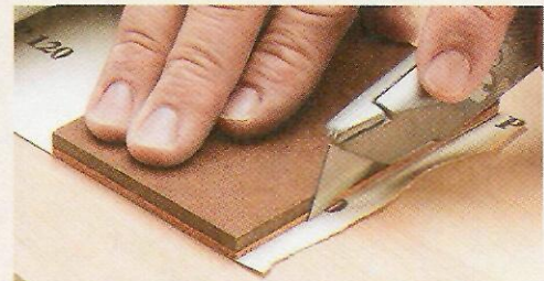
▲ Size the Sandpaper. After sticking an oversized piece of sandpaper to the pad, use a utility knife to trim the edges flush.
