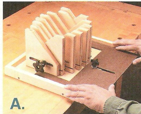
◀ Set Up Jig. To square up the V-block, place it on the base of the jig and loosen the knob that holds down the plate.
