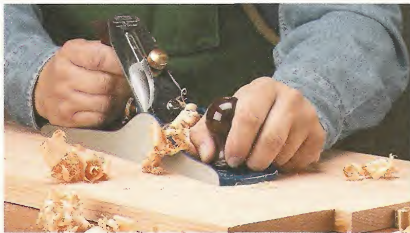
▲ Jack Plane. A jack plane like this #5 can be used to quickly flatten a glued-up panel. Once the panel is level, you can use a smoothing plane (#3 or #4) to remove any planing marks left behind by the jack plane.
