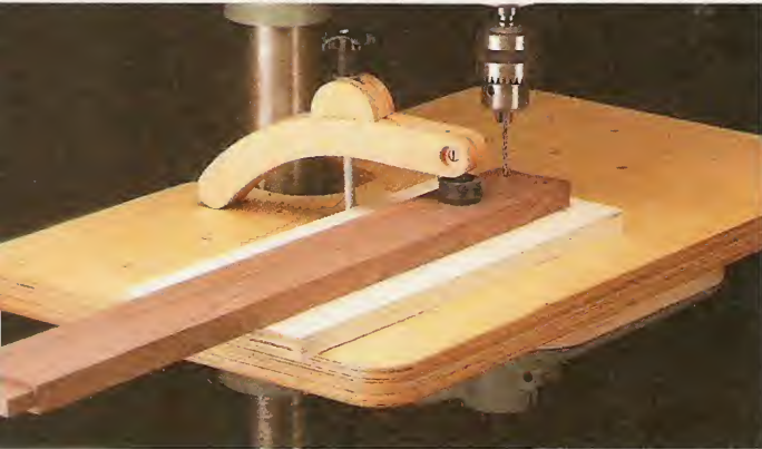
▲ Drill Press Table. This drill press table and hold-downs can be used with or without the V-block.
