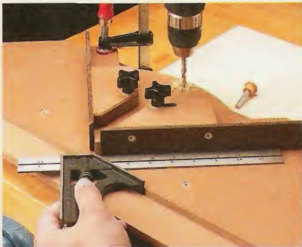
1 To drill the holes in the base for the locking pin, use a square to position the stop block. With the stop block clamped in place, drill a hole in the base, using the hole in the stop block as a guide.
