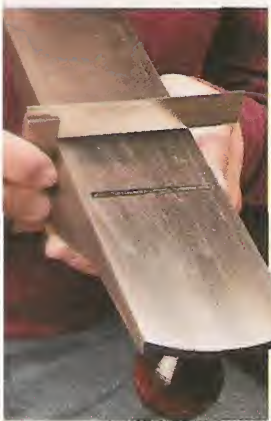
▲ Check for Square. To get good results, the sides of your plane need to be square with the sole.
