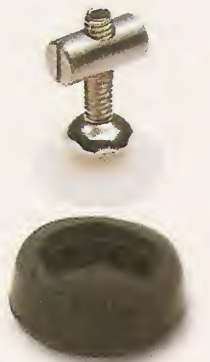
▲ Clamp Pad. To make the clamp pad, thread a leg leveler into a barrel nut. Then cut off the end of a rubber crutch tip and slip it over the leg leveler.
