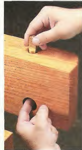
▲ Finger Holes. Access holes drilled on the inside face of the vise make it easy to "pop up" a bench dog for easy removal.
