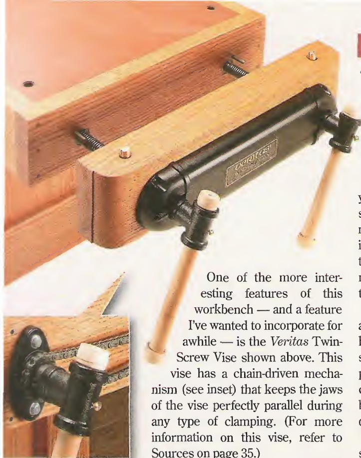
▲ With the vise cover removed, you can see the chain-drive mechanism that operates the vise.
