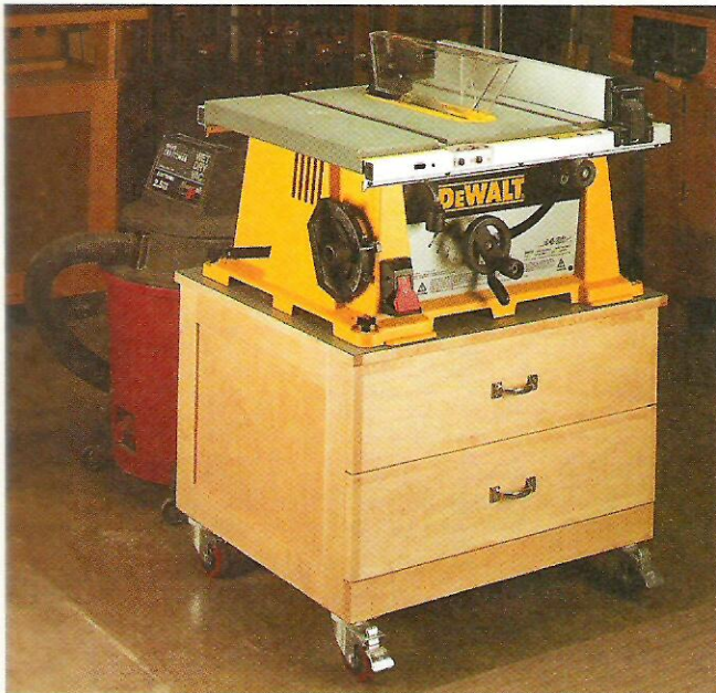
▲ Saw Cabinet. As a stand-alone unit, the saw cabinet provides solid support for a portable saw with plenty of storage for accessories.
