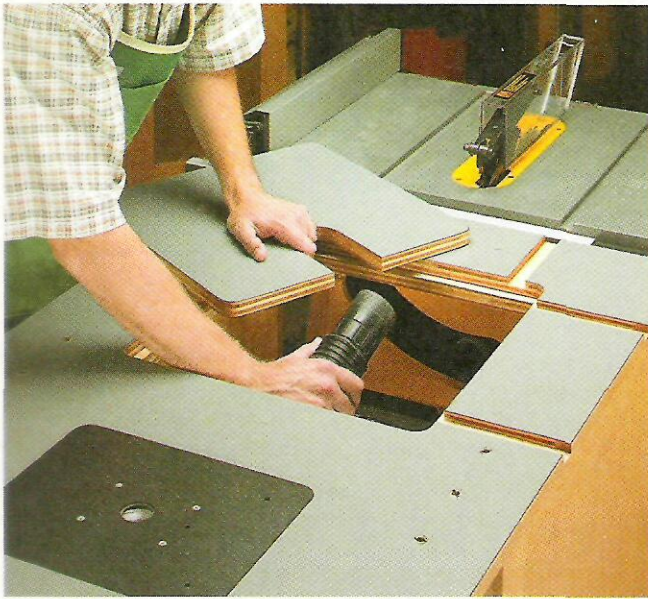
▲ Access Panel. Just "pop out" the panel from the top of the outfeed cabinet to provide easy access to the shop vacuum inside.
