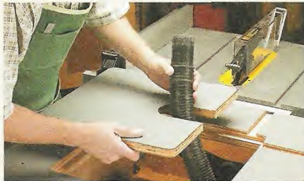
B. Shop Vacuum Access. A removable panel provides quick access when hooking the dust hose from the shop vacuum up to the table saw or router table fence.
