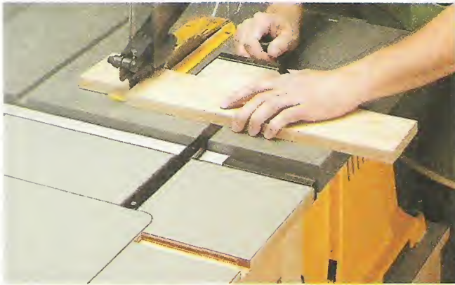
▲ Miter Slots. Routing slots in the top of the outfeed table provides clearance for the bar of the miter gauge when making crosscuts.
