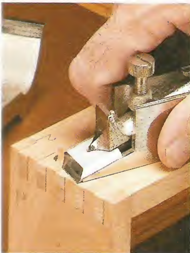
▲ Chisel Plane. With the top removed, this plane is quickly converted into a chisel plane. The low-angle blade cuts right through the end grain on this box joint.
