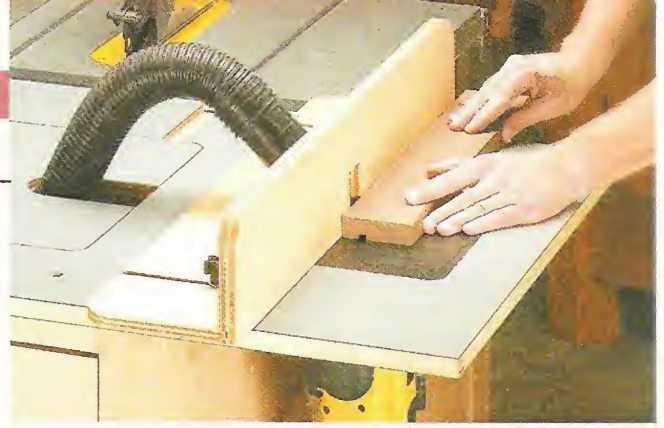
▲ Fence. Adding a fence to the router table adds versatility and allows you to hook up the hose from the shop vacuum.
