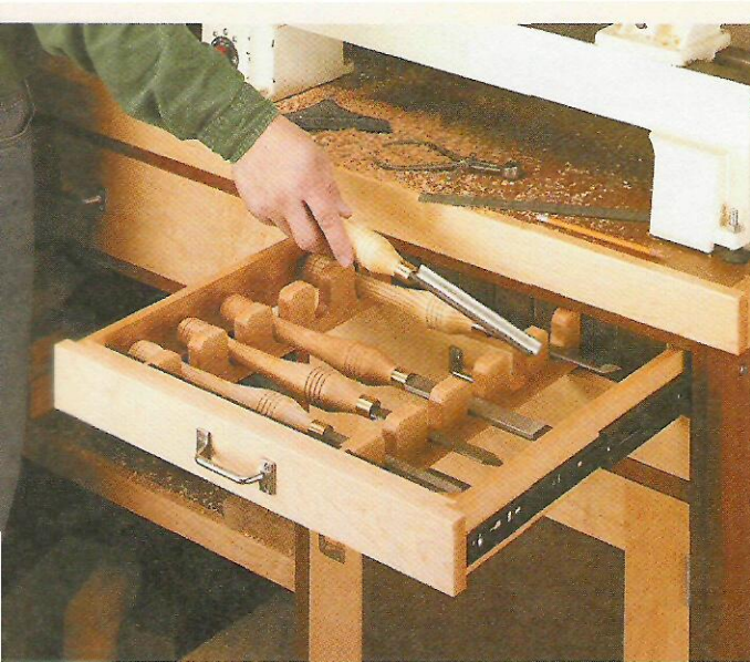
▲ Tool Storage. The two smaller drawers pull out to become a pair of handy tool racks.
