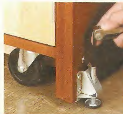
▲ Casters and Levelers. An Allen wrench is all you need to level the stand and raise the casters up off the floor.
