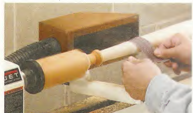
▲ Dust Hood. Hooked up to a shop vacuum, this dust hood does a great job of picking up the fine dust that is created while sanding a project on the lathe.
