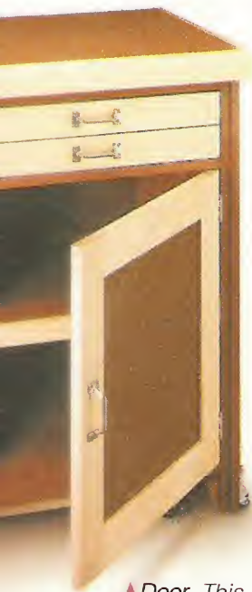
▲ Door. This door keeps chips and debris from collecting inside the storage area.
