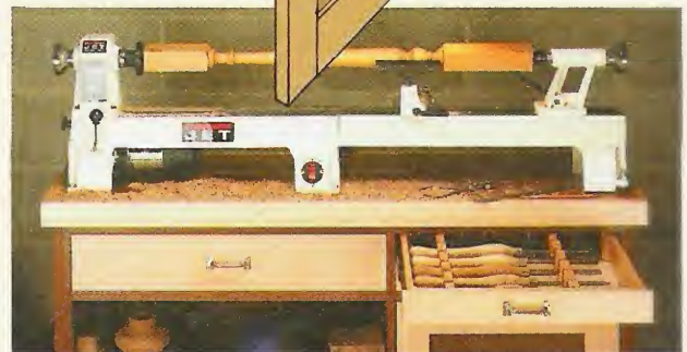
▲ Bed Extension. The lathe stand is extra-long in case you decide to expand your turning capacity by adding a bed extension to your mini-lathe.
