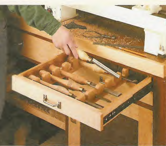
▲ Tool Storage. The two smaller drawers pull out to become a pair of handy tool racks.
