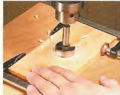
◀ Finger Openings. Clamping a pair of drawer fronts together provides solid support when drilling the circular cutouts for the finger openings.
