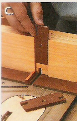
▲ Hardboard & MDF. Smooth and strong, hardboard (left) makes a fine, low-profile base or replaceable inserts. MDF (right) is an inexpensive way to build an entire jig.
