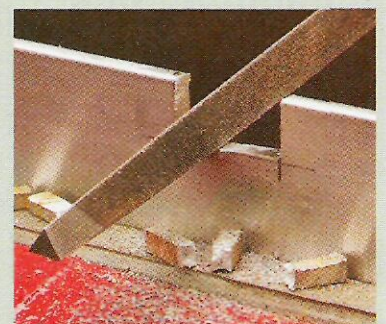
▲ File. Finally, smooth out the bottom and sides of the notch with a narrow, triangular file.
