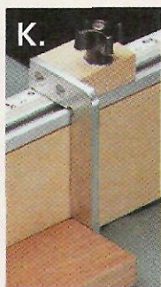
▲ Aluminum. Whether it's just a piece of flat stock for a stop block (left) or a piece of angle for the body of a shop-made tool like the scratch stock (right), aluminum is easy to use and work with.
