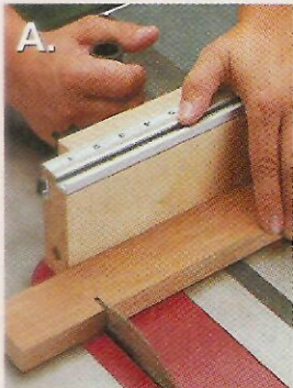
▲ Plywood. A mainstay for long-lasting jigs, high-quality plywood (like the Baltic birch shown above) provides flatness and stability for fences (left) and bases (right).
