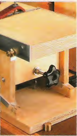
▲ Height Adjustment. Turning a knob at the end of the tapered bed will raise or lower the sliding table.
