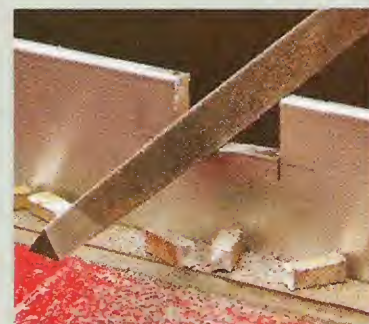
▲ File. Finally, smooth out the bottom and sides of the notch with a narrow, triangular file.
