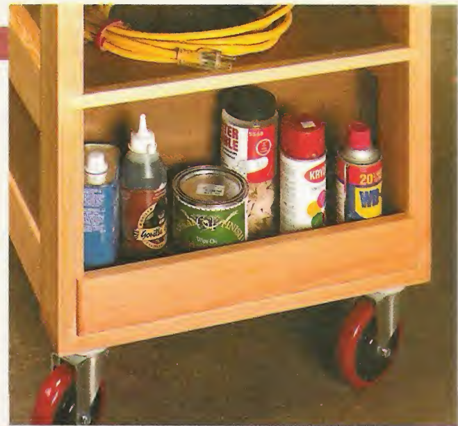
▲ Storage Cubby. Adding a "false front" to the opening at the back of the cart creates a handy storage area for often-used items.
