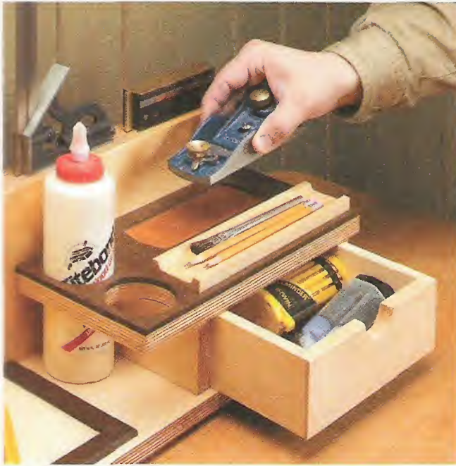
▲ Drawer and Shelf. Increase the storage options by further customizing the organizer. A drawer and shelf hold small tools, pencils, and a glue bottle or two.
