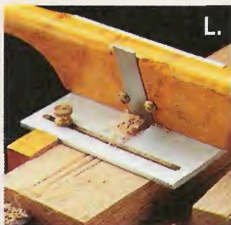
▲ Aluminum. Whether it’s just a piece of flat stock for a stop block (left) or a piece of angle for the body of a shop-made tool like the scratch stock (right), aluminum is easy to use and work with.
