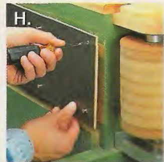
▲ Phenolic & Laminate. A phenolic plate is the perfect choice for mounting a router (left). And laminate makes a long-wearing and easily replaceable platen for an edge sander (right).
