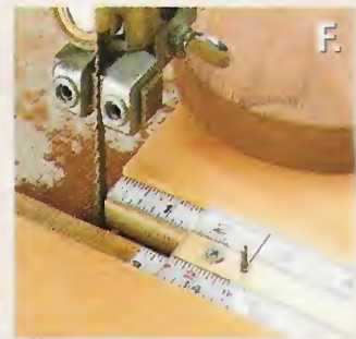
▲ Polycarbonate & Acrylic. Virtually unbreakable, polycarbonate is best for see-through guards (left) while inexpensive acrylic makes a great hairline indicator (right).
