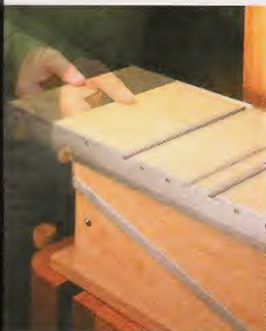
▲ Sliding Table. To rout a mortise, the table slides from side to side on the tapered bed.
