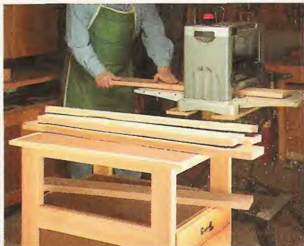
▲ Multiple Worksurfaces. Whether you're working at the table saw, jointer, or planer (shown above), the lower shelf is the perfect place to store completed workpieces.
