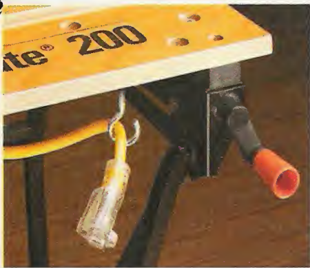
▲ Dana Craig of Norwood, MA keeps an extension cord within arm's reach by slipping the cord through a partially opened eyebolt attached to his Workmate.
