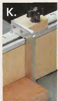
▲ Aluminum. Whether it’s just a piece of flat stock for a stop block (left) or a piece of angle for the body of a shop-made tool like the scratch stock (right), aluminum is easy to use and work with.
