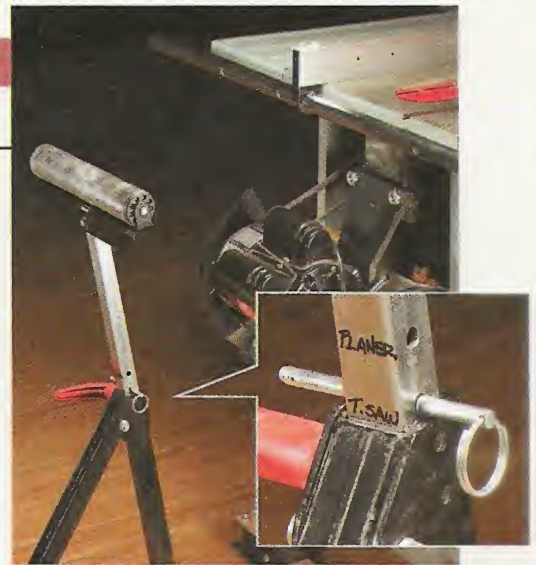
▲ Mark McConnel of Costa Mesa, CA quickly sets the height of his outfeed rollers by drilling holes in the riser and locking it in place with a hitch pin.
