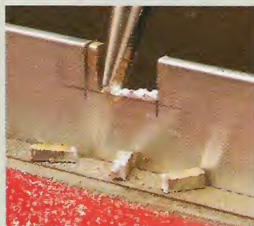
▲ Snap. Using a pair of needle-nose pliers, snap off the remaining waste pieces one by one.
