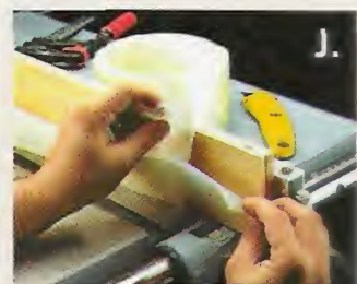
▲ UHMW. Jigs slide easily when they’re guided by a runner (left) made from UHMW. And a workpiece will slide just as easily by adding a thin strip of UHMW (right) to an auxiliary fence.
