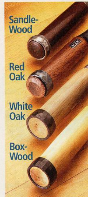
▲ Handle Choices. These are the most common hardwood handles found in Japanese chisels.
