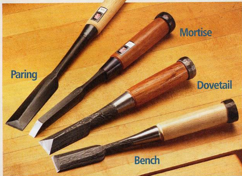
▲ Types of Chisels. Japanese chisels come in a variety of styles depending on their use. Bench chisels (bottom) are designed for everyday work. Long-handled paring chisels (top) are designed for pushing only.
