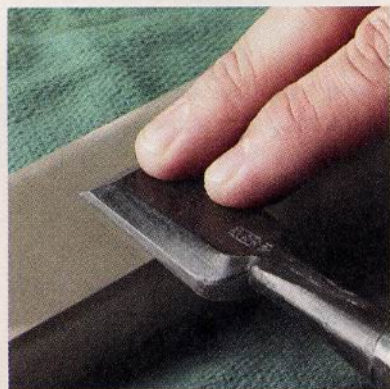
▲ Flatten the Back. Lap the back of the chisel on waterstones to make sure the back is flat.
