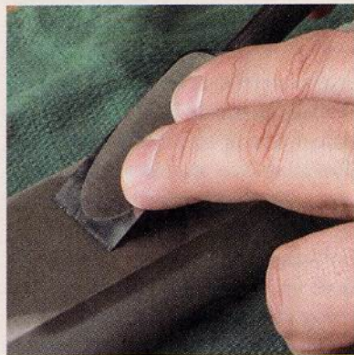
▲ Honing the Bevel. Most Japanese chisels won't fit in a jig, so you'll have to hone the bevel by hand.
