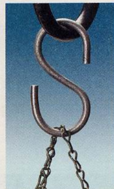
▲ S-Hooks. We bent this S-hook out of a piece of 3/16"-dia. steel rod.
