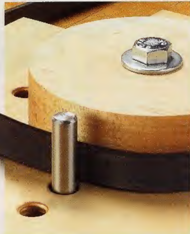
Wheel. To create perfect arcs, a wooden wheel is used as a bending form. The metal is held in place by a steel pin during the bending.
