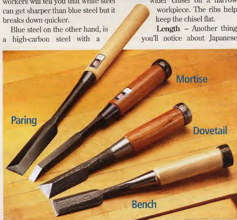
▲ Types of Chisels. Japanese chisels come in a variety of styles depending on their use. Bench chisels (bottom) are designed for everyday work. Long-handled paring chisels (top) are designed for pushing only.
