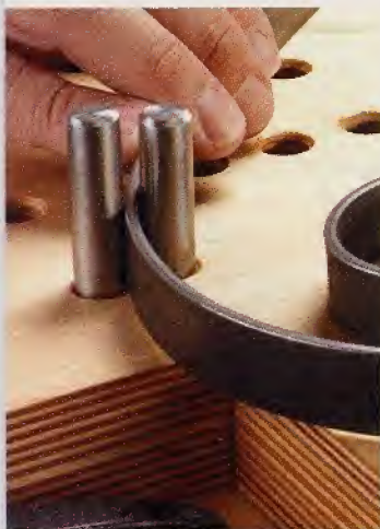
▲ Pins. To create freehand bends, the metal is bent between a pair of steel pins.
