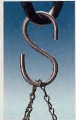
▲ S-Hooks. We bent this S-hook out of a piece of 3/16"-dia. steel rod.
