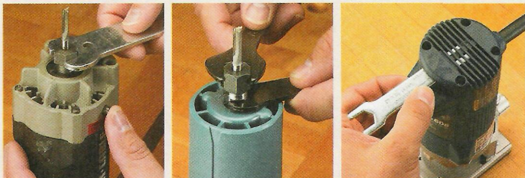
▲ Bit Changes. Like some full-size routers, trim routers that use a single wrench with a spindle lock wrenches can be easier to use, whether both wrenches are used at the collet (center photo) or one slips into the top of the router (right photo).
