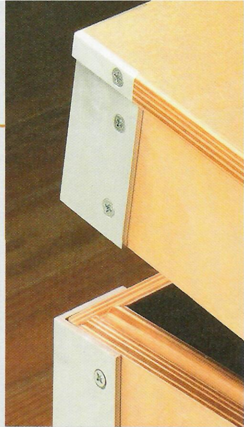
▲ Aluminum Angle. Ordinary aluminum angle reinforces the corners of the gear box. Besides protecting them from wear and tear, the aluminum angle provides a striking look.
