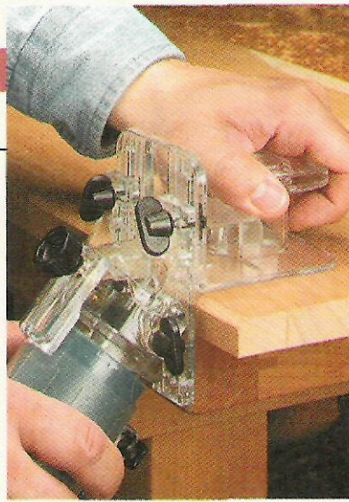
▲ Base Attachment. The attachment shown on the Makita trim router works with the tilting base to rout chamfers with a straight bit.
