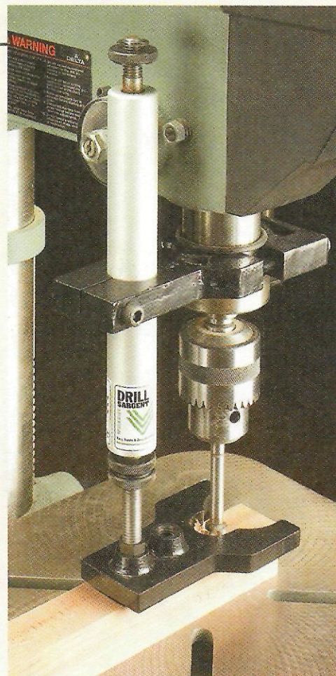
▲ Drill Sargent. This add-on accessory uses a spring-loaded foot to hold down the workpiece. The foot automatically lifts as you raise the drill bit out of the hole.
