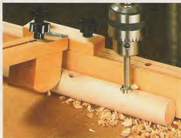
▲ Dowels. The convex shape of the bottom of the hold-down block allows you to firmly grip dowels or other odd-shaped workpieces while drilling holes.
