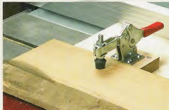
▲ Overhead. The end of this toggle clamp has a rubber "foot" that grips the workpiece without slipping. It can be adjusted for different thicknesses of stock.
