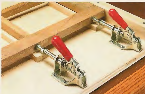
▲ In-Line. These in-line toggle clamps are perfect for holding a door frame in this assembly jig. Each one is capable of applying 300 lbs. of clamping force.
