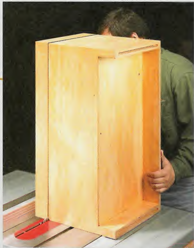
▲ Separating a Lid from a Case. After cutting completely through the long sides of the case, lower the saw blade and "score" the short sides to almost separate the lid from the case.
