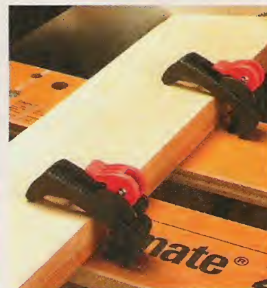
▲ Cam. These plastic-bodied hold-downs use a cam-locking device to apply pressure to the workpiece.
