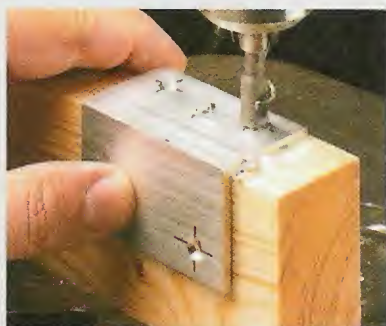
▲ Cutting, Drilling, & Routing. An auxiliary fence attached to your miter gauge supports the workpiece when making a cut with a carbide-tipped saw blade. After you've cut all the pieces to length, drill and countersink
