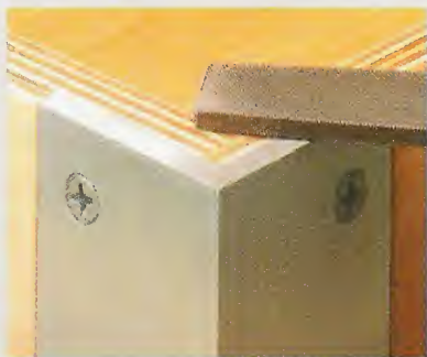
▲ Finishing Touches. To smooth the cut edges of the aluminum angle (and flush the ends with case and lid), use a mill file. Once that's complete, you can remove the aluminum angle and sand the surfaces
