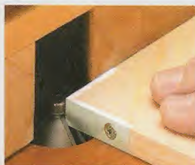
▲ Aluminum Angle. Ordinary aluminum angle reinforces the corners of the gear box. Besides protecting them from wear and tear, the aluminum angle provides a striking look.
