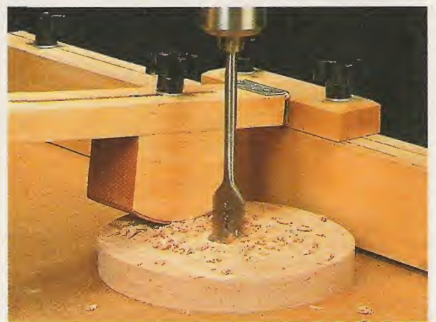
▲ Small Workpieces. The hold-down easily holds small workpieces, allowing you to keep your hands a safe distance from the drill bit.
