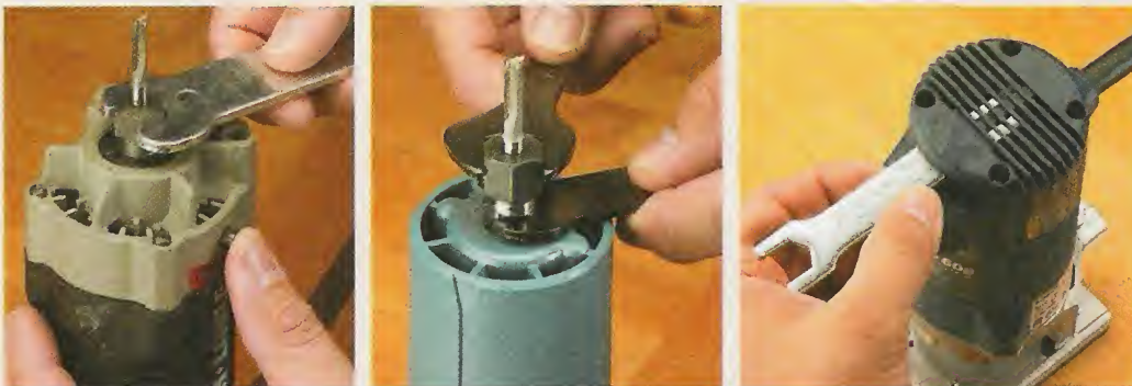
▲ Bit Changes. Like some full-size routers, trim routers that use a single wrench with a spindle lock wrenches can be easier to use, whether both wrenches are used at the collet (center photo) or one slips into the top of the router (right photo).
