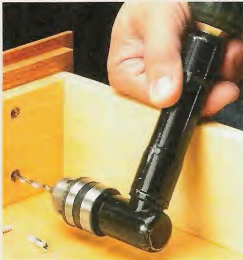
▲ Drill at an Angle. A right-angled drive attachment is invaluable when you need to drill or drive a screw in a tight spot.
