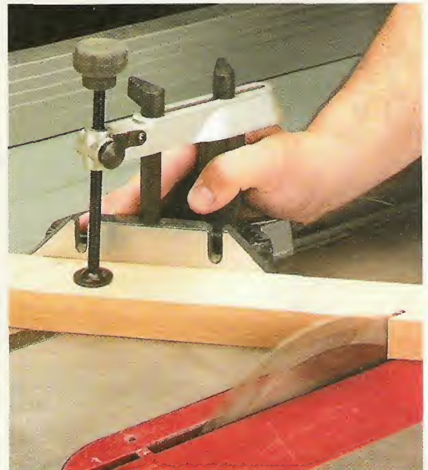
▲ Small Workpiece Hold-Down. Although it only has one clamp screw and lacks the capacity of the Delta version, this Sears miter gauge hold-down accomplishes the same thing.
