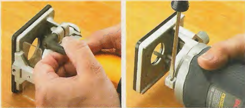
▲ Removing the Base. Getting clear access to the bit or collet almost always requires removal of the base. A tool-free, quick-release lever minimizes the hassle, unlike a trim router that requires a screwdriver.
