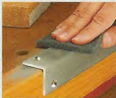
▲ Finishing Touches. To smooth the cut edges of the aluminum angle (and flush the ends with case and lid), use a mill file. Once that's complete, you can remove the aluminum angle and sand the surfaces
