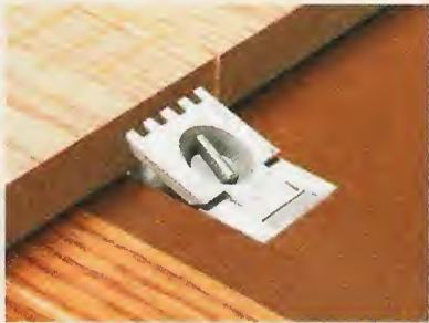
▲ Bench Stop. While it doesn't actually hold the workpiece, a stop is handy for sanding or planing.
