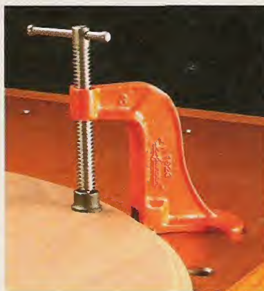
▲ Screw. This hold-down uses a simple clamp-type screw to hold the workpiece down to the bench.
