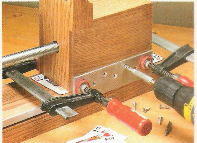
▲ A Winning Hand. Ordinary playing cards act as shims during the installation of the rails to create the necessary clearance between the base and the rear jaw.
