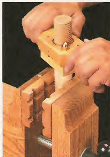
Prismatic Jaws. The V-grooves in this pair of jaw faces allows you to hold dowels or round stock either horizontally or vertically.
