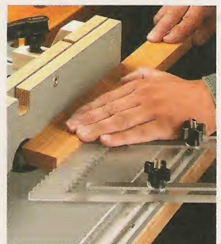
▲ Accessories. An aluminum track allows the use of a miter gauge or the featherboard shown above.
