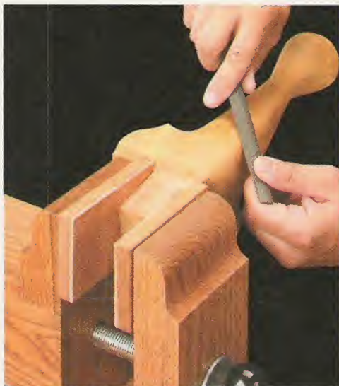
Soft Jaws. For holding delicate objects (like carvings), these leather-lined jaws provide a firm but non-marring grip.
