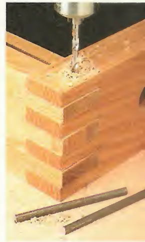
▲ Pinned Box Joint. To strengthen the box joint, I added a pair of steel rods to act as reinforcing pins.
