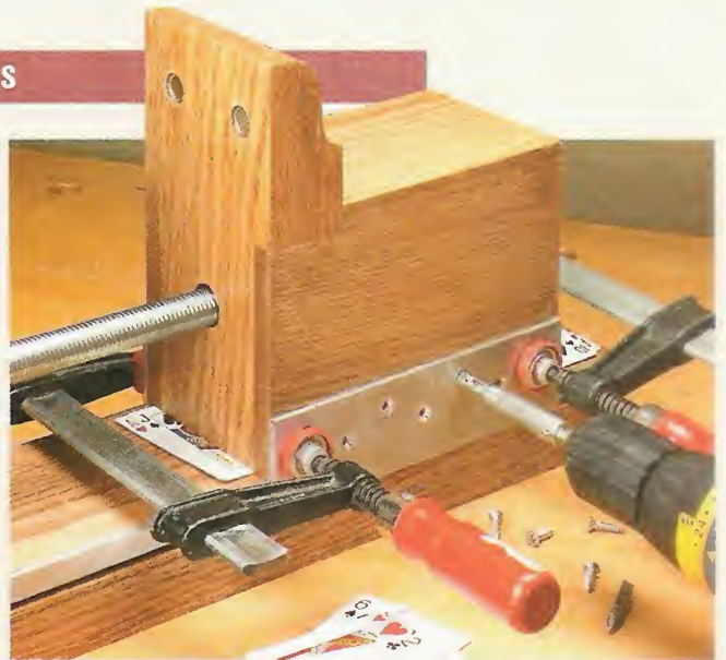
▲ A Winning Hand. Ordinary playing cards act as shims during the installation of the rails to create the necessary clearance between the base and the rear jaw.
