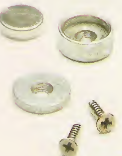
▲ Rare-Earth Magnet. This rare-earth magnet is mounted in a steel cup to increase its strength. The washer gets mounted to a removable jaw face.
