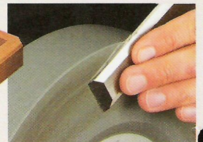
▲ Flattening the Back. Unlike a typical stone, you can use the Tormek to flatten the back of a tool.
