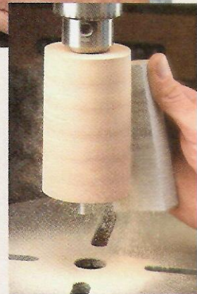
▲ Sanding the Rollers. Each roller is mounted in the drill press and sanded lightly to smooth out the rough surface left behind by the router.
