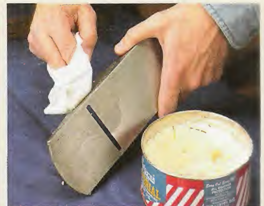
4 To help prevent future rust from forming, dry the tool thoroughly and then apply a coat of paste wax to all the bare metal surfaces.
