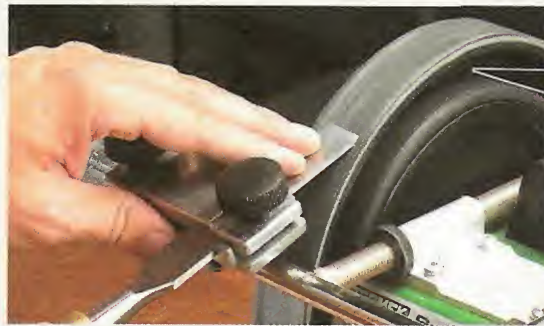
◀ Honing. After applying honing compound (see inset), the leather wheel makes quick work of polishing the edge.
