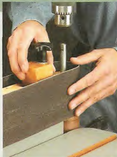
▲ Belt Change. To install or remove the sanding belt, loosen the knob and lift up the wedge to release the tension on the sanding belt.
