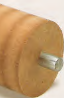
▲ Rollers. The rollers for the belt sander are built up out of several layers of MDF. Then they're trued up using a router table and jig (see opposite page).
