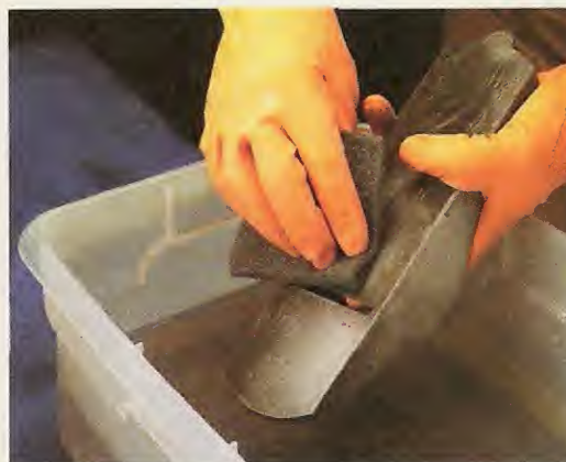
3 Once the electrolysis is complete, rinse the tool off in clean water and scrub the surfaces gently with the abrasive pad.
