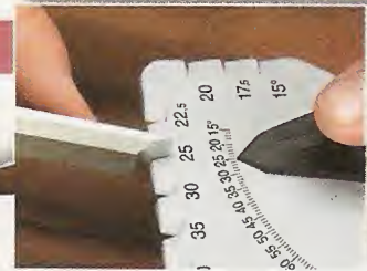
◀ Set the Angle. With the AngleMaster, you can verify (see inset) and set the sharpening angle perfectly.
