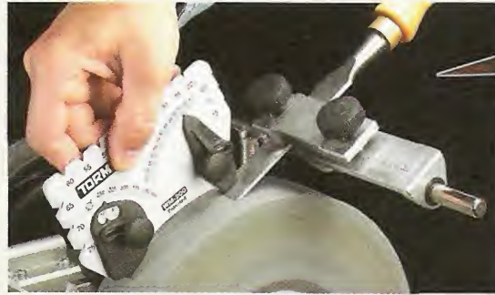
◀ Set the Angle. With the AngleMaster, you can verify (see inset) and set the sharpening angle perfectly.
