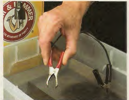
2 With the battery charger unplugged, clamp the negative lead to the tool and the positive lead to the anode (a scrap piece of steel).
