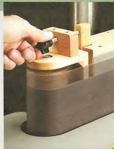
▲ Tracking. Turning a knob at the end of the sander will cause the idler roller to pivot slightly, thereby centering the belt.
