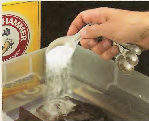
1 To get started, mix a tablespoon or two of washing powder in a plastic tub filled with enough water to cover the top of the tool.
