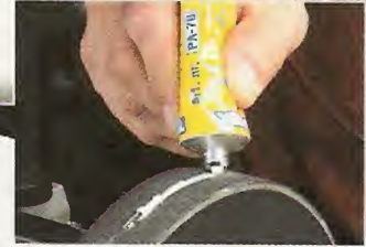
◀ Honing. After applying honing compound (see inset), the leather wheel makes quick work of polishing the edge.
