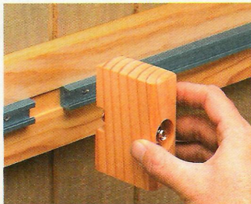
▲ Gap. For extra-long runs of track, you can leave a space in between the aluminum T-tracks to make inserting the blocks easier.
