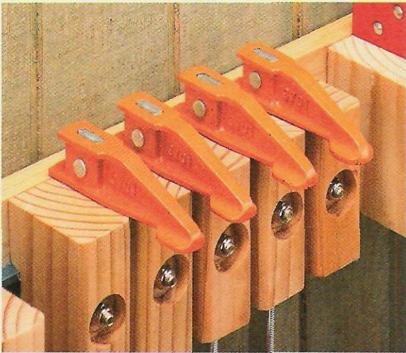
▲ Narrow Blocks. The basic block is fastened to the T-track with a toilet bolt, a washer, and a nut. Grouping the blocks together makes slots for holding bar clamps.
