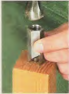
▲ Drive Center. A few taps with hammer is all it takes to embed the drive spurs in the workpiece.
