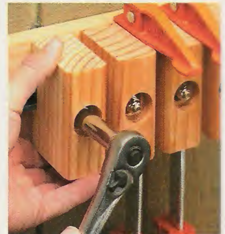
▲ Lock-Down. All it takes to reconfigure the clamp storage system is a ratchet with a 7/16" socket.
