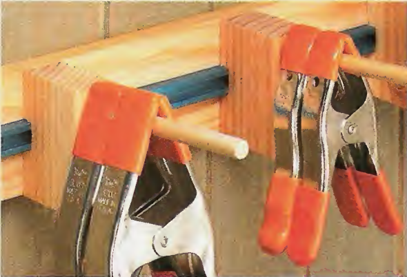
▲ Peg Blocks. By gluing a dowel in an angled hole drilled in a block, you can make a handy place to keep spring clamps. Two peg blocks side-by-side can be used to hold C-clamps in place.
