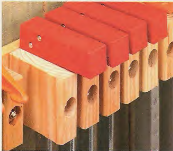
▲ Wide Blocks. To accommodate large, heavy-duty clamps like the parallel jaw clamps shown here, the basic block can be made a little wider.
