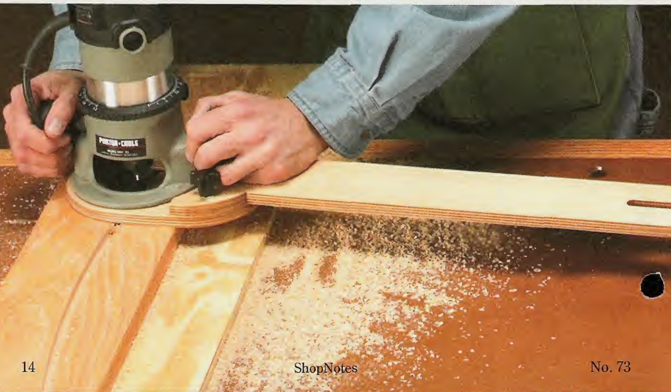
FIRST: CARPET TAPE WORKPIECE TO SCRAP PIECE, THEN CLAMP TO WORKBENCH
