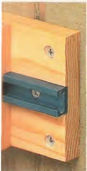
▲ T-Track. Each section of track consists of an aluminum T-track fastened to a wall plate. The sections are then screwed to the wall studs.
