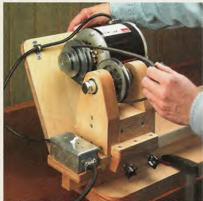
▲ Changing Speed. With the motor mounted to a hinged platform, shifting the belt to change the lathe speed is just a matter of lifting the back end of the mount. After adjusting the belt, swing the platform back down to reapply tension.
