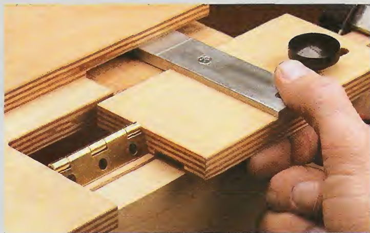
1 To set the length of the mortise, you can use the hinge to position the two parts of the base. Just be sure the inside edge of each base contacts the leaves of the hinge.
