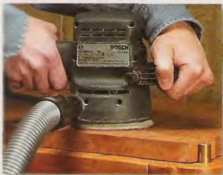
▲ Dust-Free. When hooked up to a major dust producer like this sander, the Fein shop vacuum virtually eliminates dust.
