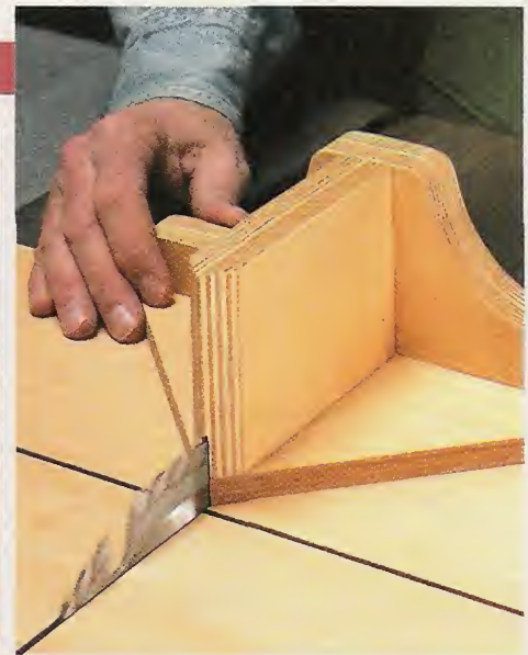
▲ Cutting a Kerf in the Sled. Once the sled is complete, you'll need to cut a kerf. To do this, raise the blade about 1 1/2". Next, push the sled through the blade (left) and complete the kerf by sliding the sled until the blade is "buried" half way into the blade housing (right).
