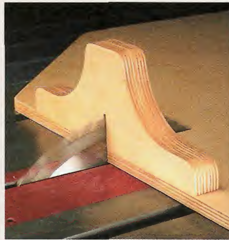
▲ Cutting a Kerf in the Sled. Once the sled is complete, you'll need to cut a kerf. To do this, raise the blade about 1 1/2". Next, push the sled through the blade (left) and complete the kerf by sliding the sled until the blade is "buried" half way into the blade housing (right).
