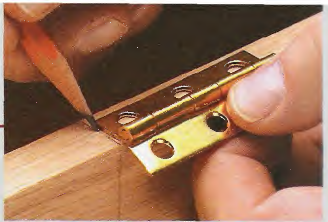
▲ Lay Out Location. The first step in routing a mortise for a hinge is to lay out the location of the hinge along the edge of the workpiece.
