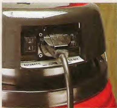
▲ The "Brains." Switched to auto mode, the vacuum powers up automatically when you turn on a tool.
