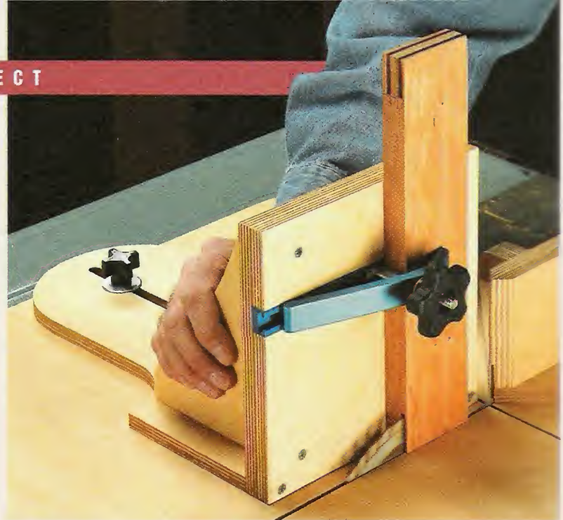
▲ Add-On Tenoning Jig. Cutting the cheeks of a tenon that are perfectly smooth is fast, easy, and accurate with the tenoning jig shown above. The jig mounts to the cut-off sled in place of the fence and features a replaceable stop and sturdy hold-down.
