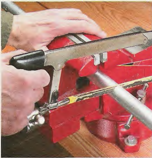
▲ Pipe Jaws. A secondary set of jaws on this vise can be used to hold pipe or rods.
