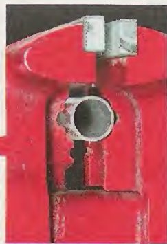
▲ Pipe Jaws. A secondary set of jaws on this vise can be used to hold pipe or rods.
