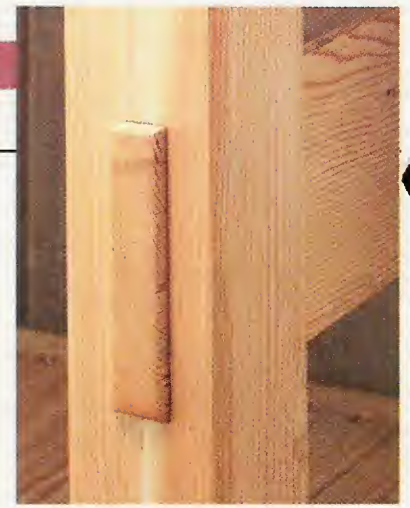
▲ Through Tenons. A few cuts on the table saw are all it takes to make perfectly sized mortises for the through tenons of the bench.
