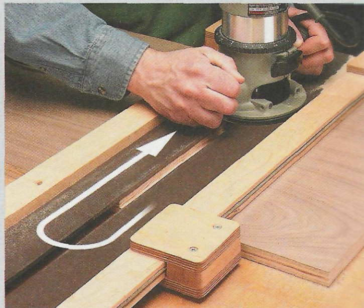
▲ Completing the Cut. For dados wider than \frac{1}{2} " , you'll need to make a second pass along the other fence of the jig. To rout the other side of the dado, turn the router around so that the arrow side is against the other fence. Then rout back to the starting point.
