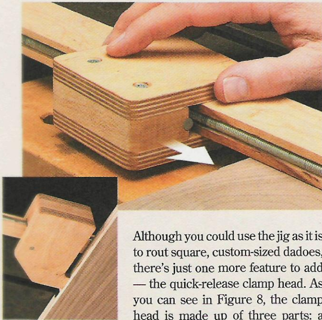
▲ Clamp Head. The self-clamping head locks the jig in place on the workpiece.
