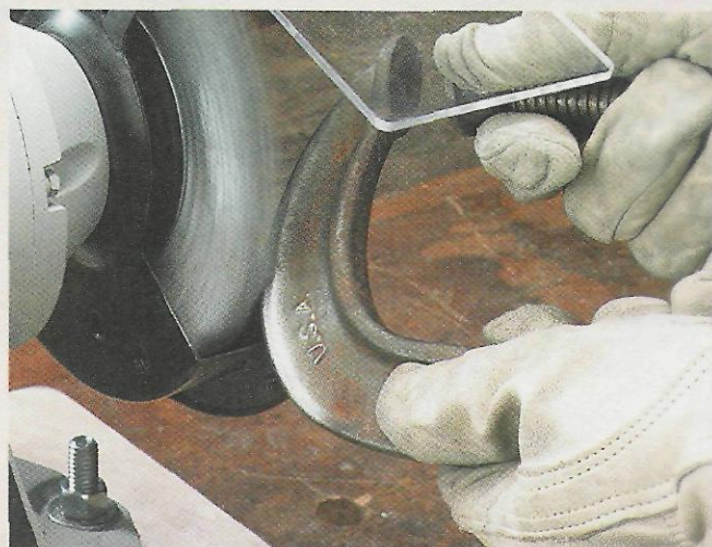
▲ Other Options. A bench grinder can do more than just remove metal. Adding a shine to a project with a buffing wheel (top) or cleaning up tools with a wire wheel (bottom) adds to a grinder's versatility.
