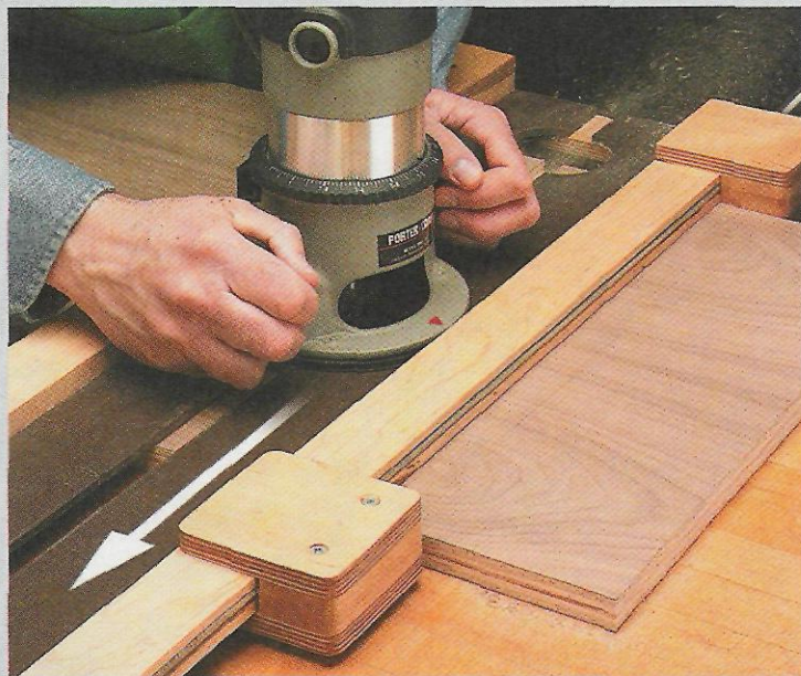
▲ Routing the Dado. For the best results, rout the dados with the same edge of the router base held against the fence rails. I drew an arrow on the router to serve as a reminder. First, rout all the way across the panel with the router against one fence.
