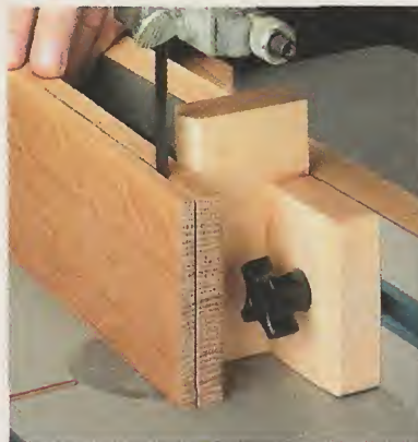
◀ Resawing. The adjustable pivot block allows you to resaw thick stock into thinner stock with precision.
