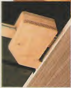
▲ Clamp Head. The self-clamping head locks the jig in place on the workpiece.
