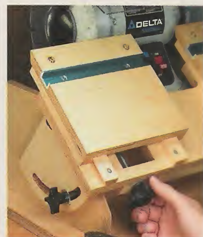
▲ Slide. To move the sliding table closer to (or further away from) the grinding wheel, turn the knob along the front of the pivoting platform.
