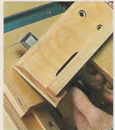
▲ Check Your Progress. You can check your grinding progress by simply turning the tool sled over.
