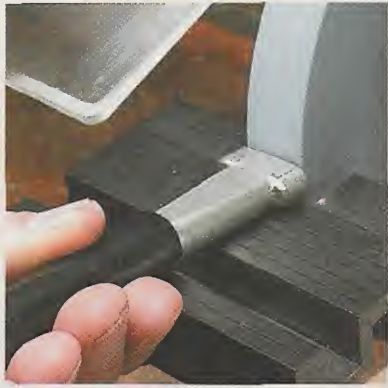
▲ Dress for Success. Removing embedded metal from the stone and truing it up with a diamond dresser ensures peak performance.
