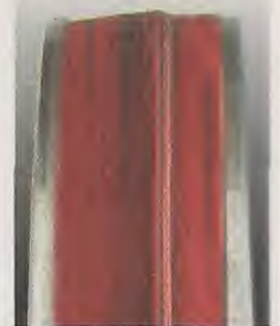
▲ Tire Wear. The ridge on this tire was caused by setting the blade tension too high.
