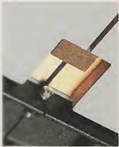
▲ Access. A small cutout in the bottom of the table provides access to the pin and hardboard key that keep the surfaces of the cast iron table and the auxiliary table aligned.
