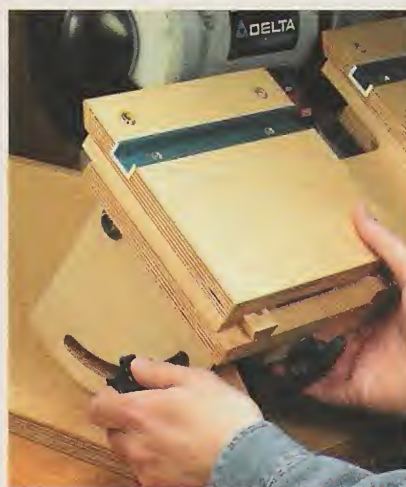
▲ Pivot. To adjust the angle of the pivoting platform, loosen the two star knobs on the sides of the wings and swing the platform into position.
