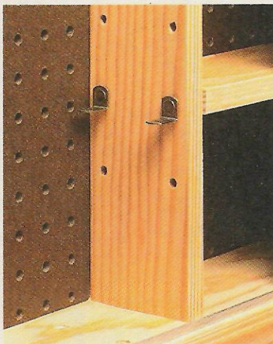
▲ Shelf Pins. Removable shelf pins are used to support the adjustable shelves inside the pegboard storage cabinet.
