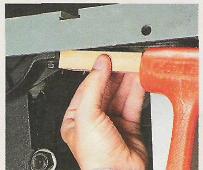
▼ A Little Tap. To align the blade with the miter slot, loosen the trunnion bolts and tap the trunnion into alignment.
