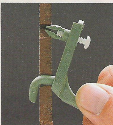
▲ Insert Hook. With the white, nylon screw backed out, slip the hook into a pair of holes in the pegboard.
