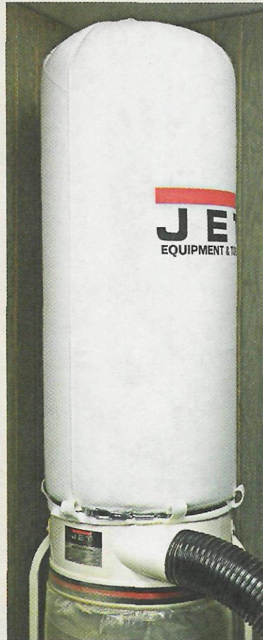
▲ Filter Bags. A finer filter bag will capture more of the small dust particles, keeping your shop cleaner and less of a health hazard.
