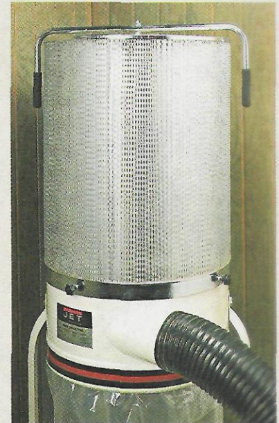
▲ Canister. The design of a canister filter (top) traps most of the dust and increases the filtering area for better overall performance.
