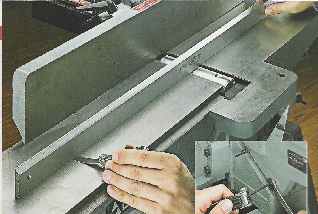
▲ Checking the Alignment. A precision straightedge and feeler gauge allow you to check whether the outfeed table sags (top). Snugging up the gib may help remove the sag (inset).
