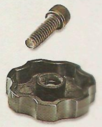
▲ Locking Knob. To make the locking knob for the layout square, a cap screw is press-fit into a blind hole in the center of the knob.
