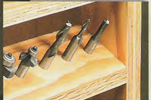
▲ Bit Rack. With the angled bit rack, you can quickly see and pick out the one you're looking for.
