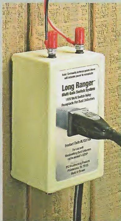
▲ Control Box. Opening a blast gate sends a low-voltage signal to this control box to automatically turn the dust collector on (or off).
