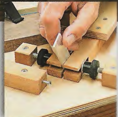
▲ Plus or Minus 45° Cuts. Whenever you need to cut an angle greater or less than 45° to square up a miter joint, simply lift up the aluminum guide stop. Then adjust the two knobs to change the miter angle for trimming.
