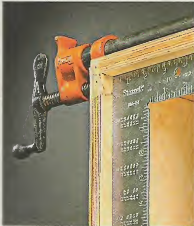
▲ Square it Up. A framing square is the perfect tool for checking large cases or frames for square.
