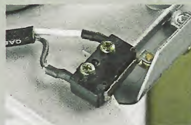
▲ Send a Signal. With the gate open (top), a microswitch "signals" the dust collector to turn on. Once closed (bottom), the collector shuts off.
