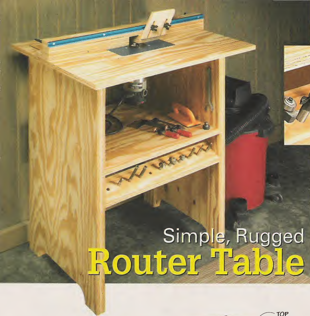
▲ Bit Rack. With the angled bit rack, you can quickly see and pick out the one you're looking for.
