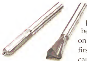
▲ Bits by the Pair. Through dovetails require a pair of bits — a dovetail bit for the tails, and a straight bit for routing the pins.
