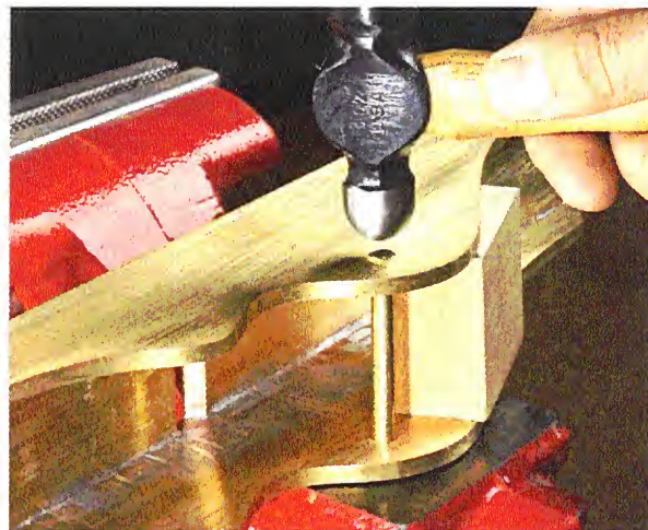
▲ Add the Pin. Cut the brass rod for the cross pin a hair longer than needed and peen the ends over with a hammer. Then file and sand the ends of the pin flush with the surface of the sides of the plane.
