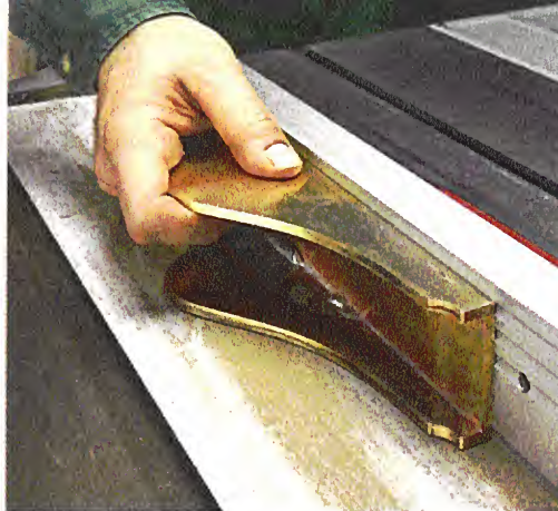
▲ Square it Up. To clean up the outside of the plane and square the sides with the sole, place a piece of adhesive-backed sandpaper on the top of your table saw.
