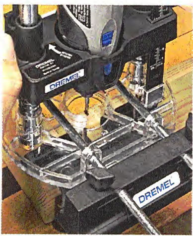
▲ Plunge Base. The plunge base and a clear plastic sub-base provide great visibility for routing out hinge mortises.
