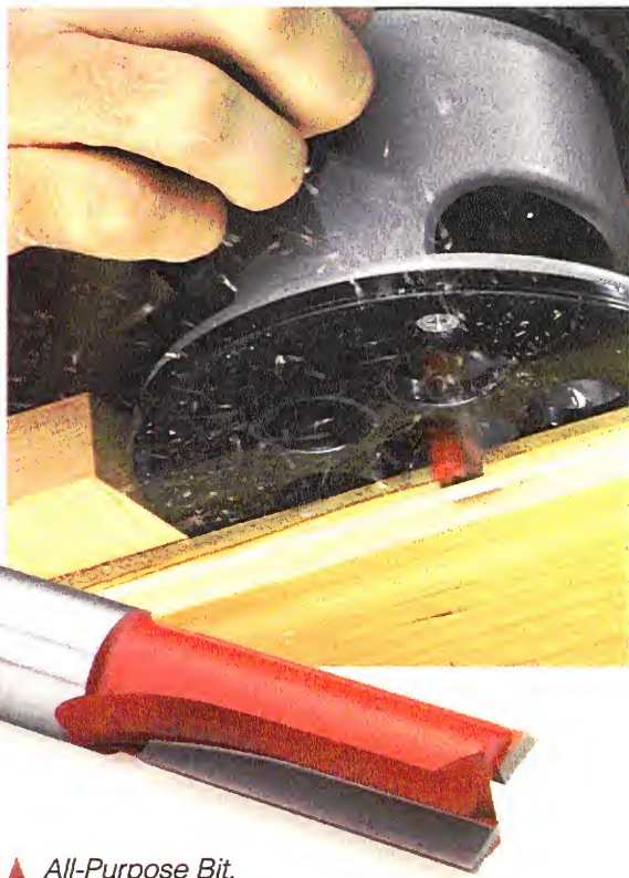
▲ All-Purpose Bit. A heavy-duty 1/2"-dia. straight bit (with 1/2" shank) will tackle most dado and grooving tasks.
