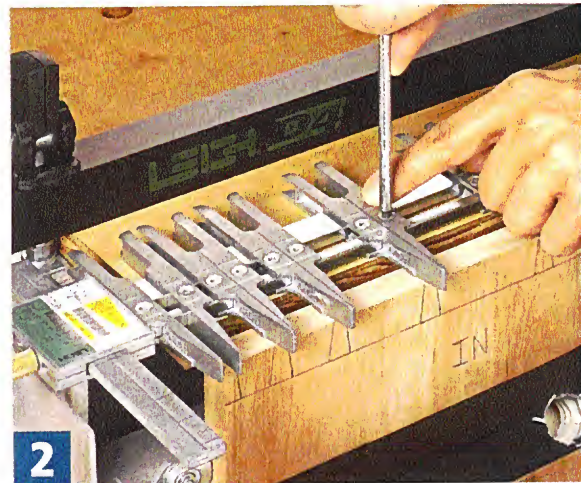
2 Adjust the Fingers. Using the tail board as a guide, adjust the fingers to match nearly any layout you can come up with.
