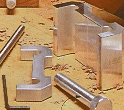
Jig can be repositioned quickly with indexing pin
