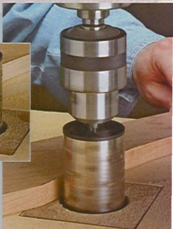
▶ Power Shaper. A Microplane drill press rotary shaper cuts faster than a drum sander and won't clog or burn the workpiece.
