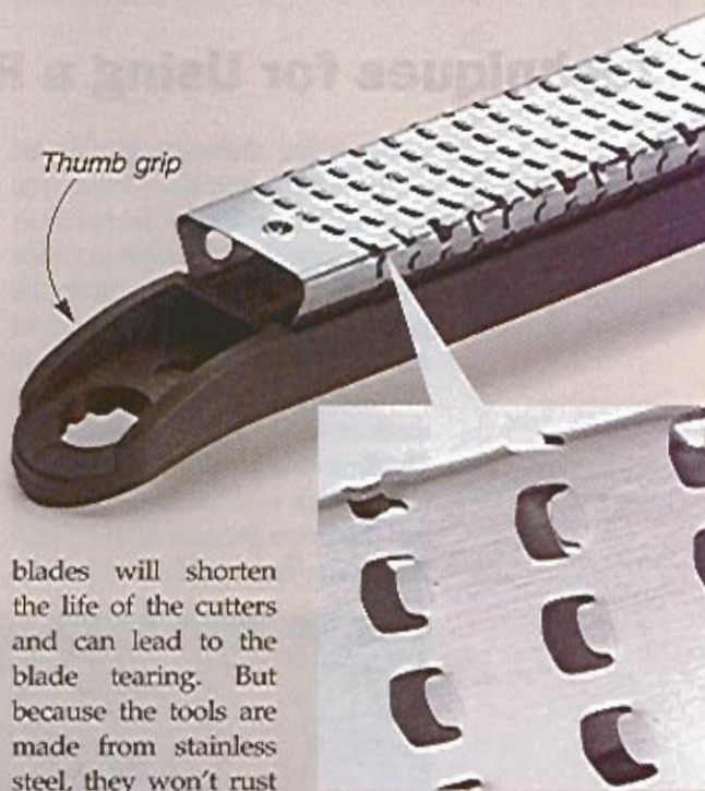
▲ Sharp Teeth. Tiny teeth are "etched" into the stainless steel blade. The non-clogging teeth slice the wood fibers cleanly.
