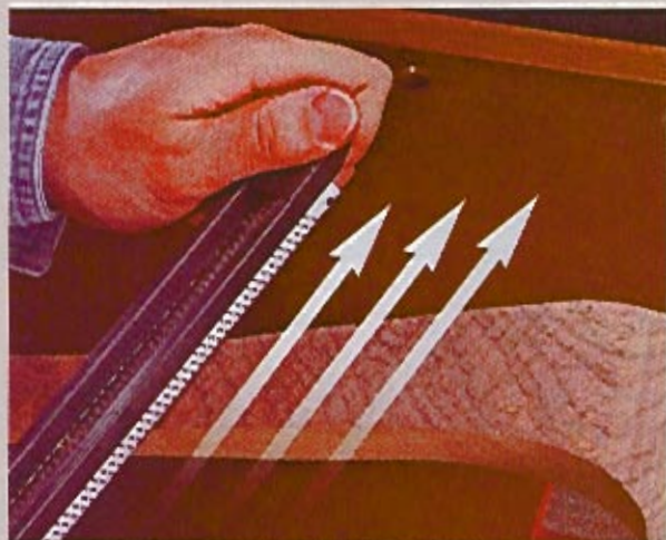
▲ Cross Strokes. Work the rasp at an angle across the grain to rough out the overall shape. The overlapping strokes will remove wood quickly.
