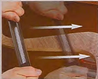
▲ Drawing the Rasp. Sliding the rasp along the workpiece removes scratches left by the previous steps and smooths out the shape.
