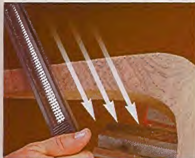
▲ The Other Way. Use cross strokes going in the opposite direction to further shape the workpiece and remove the marks from the previous step.
