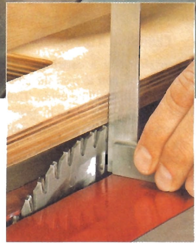
▲ Flush with the Blade. A square can take some of the guesswork out of adjusting the fence.
