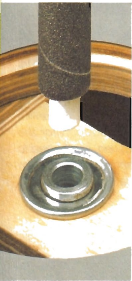
▲ Solid Support. To support the bottom of the sanding drum, the nylon spacer fits into a flange bearing.
