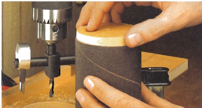
▲ Size the Disks. The first step in building a sanding drum assembly is to use a circle cutter to size the MDF disks so they just slip inside the sanding sleeve.
