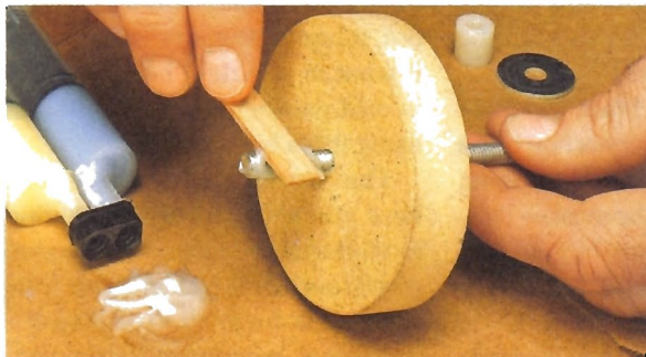
▲ Assemble the Drum. To assemble the drum, start by gluing a washer and MDF disk in place near the end of the drive shaft. Then screw the nylon spacer in place.
