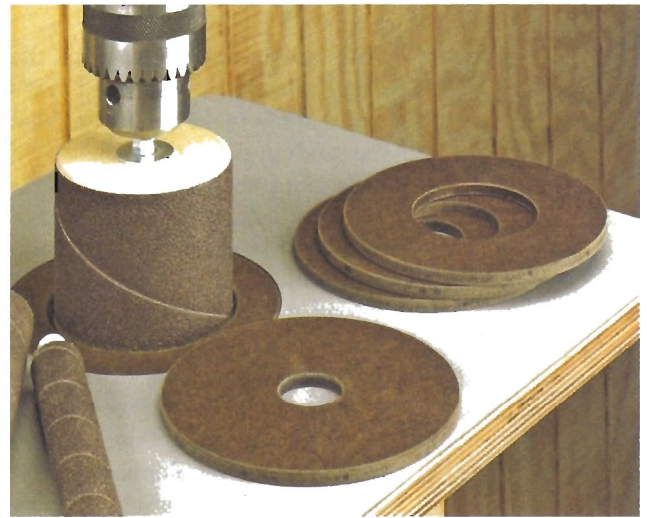
▲ Custom-Fit Inserts. To provide solid support for the workpiece and ensure good dust collection, you'll need to custom fit each insert to the table and sanding drum. To learn more about how to do this, turn to page 15.
