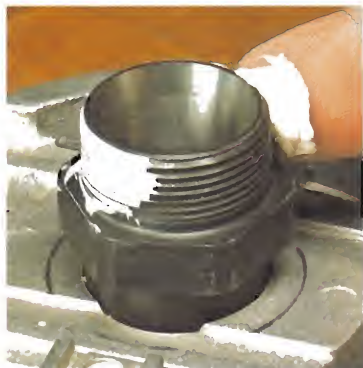
▲ Thread Lubrication. Lubricating the arbor threads makes it easier to loosen and tighten the collet nut.
