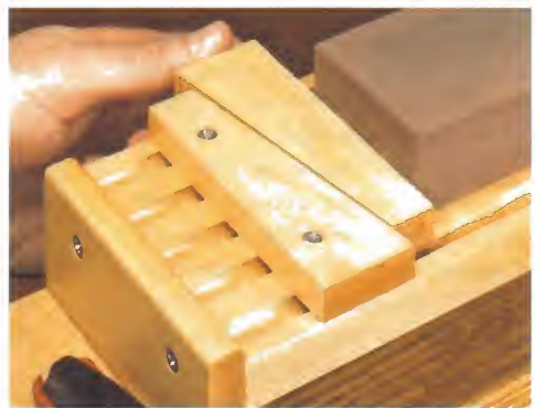
▲ Wedges Hold the Stone Tight. A pair of wedges hold the sharpening stone tightly against an adjustable cleat at the other end.
