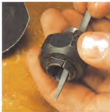
▲ Burr Removal. Small burrs inside the collet can be carefully removed using a small, half-round file.
