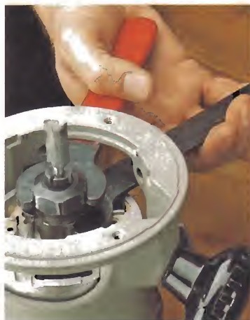
▲ Tighten Collet. Position one wrench (red handle) on the right side with the other wrench to its left. Then squeeze with one hand.
