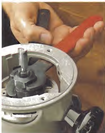
▲ Loosen Collet. Place one wrench (red handle) on the left side and the other wrench to its right. Then squeeze the wrenches together.
