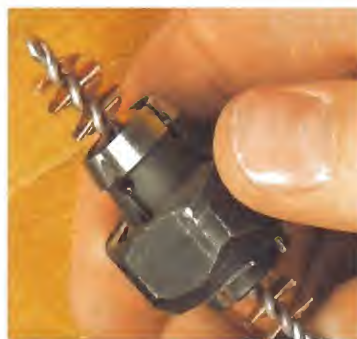
◀ Clean the Collet. Gently push a brass wire or nylon brush through the opening to remove debris from the collet.
