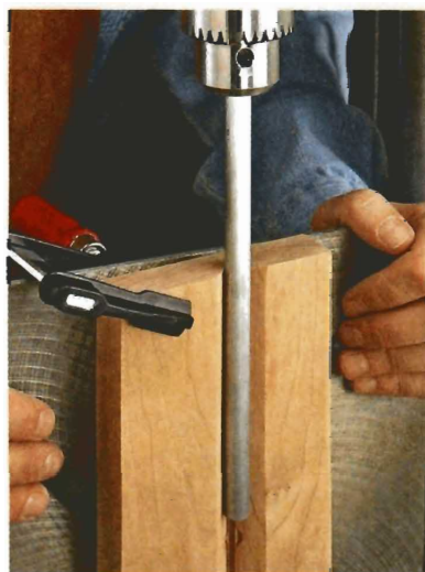
▲ Aligning the V-Block. Chuck the aluminum dowel in the drill press to set the table and V-block in place.
