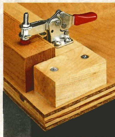
◀ Hold-Down. Toggle clamps hold the workpiece securely, allowing you to keep your fingers clear of the blade.
