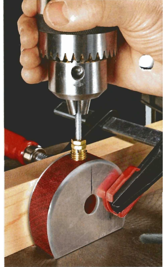
▲ Threaded Insert. After drilling the hole, use the drill press to drive in the insert into the fence.
