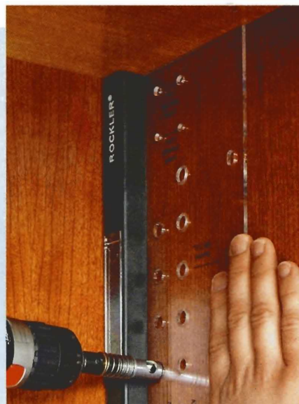
▲ After Assembly. The edge of the jig butts against the case back and top for drilling inside an assembled case.
