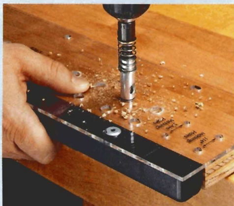
▲ Before Assembly. Use the fence to register the jig along the edge and then drill the holes with the outside row.
