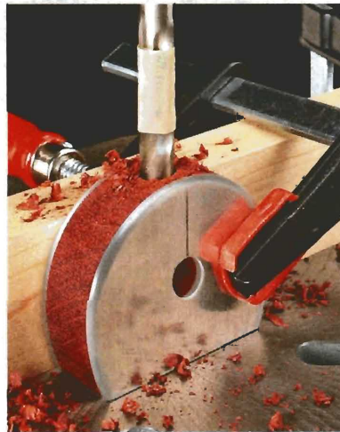
▲ Drilling the Fence. Secure the fence and drill a hole in the top to the hole in the face of the fence.
