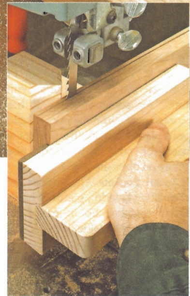
▲ Complete Control. A shop-made push block allows you to safely feed the workpiece through the end of the cut.
