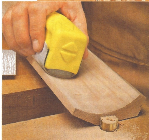
◀ Easy Sanding. The adjustable profile sander shown at left, makes easy work of smoothing the cove cut.
