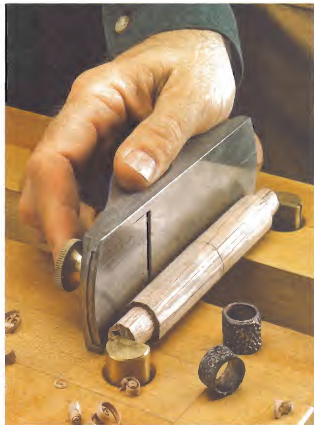
▲ The Final Touch. Starting from the center, taper the handle toward both ends using a block plane to create a faceted, barrel shape.
