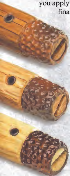
◀ No Oil. Heating the ferrules with no oil on them simply gives the copper an antique look.
