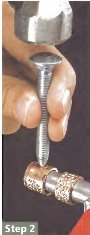
▲ Dimples. Randomly tap the bolt to add "dimples" to the ferrules. I had to file the end of the steel rod a little to get the bushing on.
