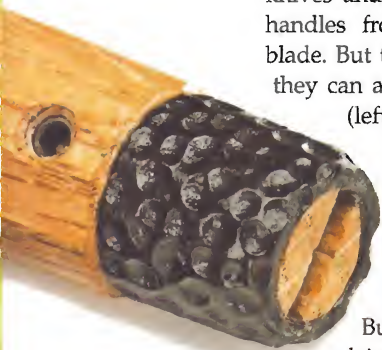
▲ Dark Finish. Burning tung oil onto the copper ferrules results in this black finish.
