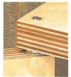
▲ Pivot Pins. A steel pin is used to mount the door. Two washers spaced between the door and the support allow the door to swing freely.
