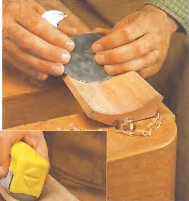
◀ Easy Sanding. The adjustable profile sander shown at left, makes easy work of smoothing the cove cut.
