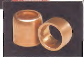
▲ Copper Ferrules. To cut the end ferrule to its final size, slide it onto a wood dowel and trim it with a hacksaw.
