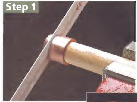
▲ Copper Ferrules. To cut the end ferrule to its final size, slide it onto a wood dowel and trim it with a hacksaw.
