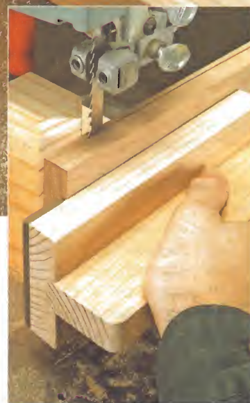
▲ Complete Control. A shop-made push block allows you to safely feed the workpiece through the end of the cut.
