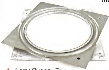
▲ Lazy Susan. The key to how well this circle jig works is an ordinary lazy Susan that allows the router to rotate.
