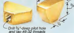
Note: Tap threads before cutting knob to shape from \frac{3}{16} " x \frac{1}{2} " bar stock
