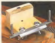
▲ A Razor-Sharp Edge. A pair of finish washers hold the blade tightly in the jig allowing you to easily hone the cutting edge.
