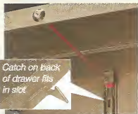
▼ Locking Drawers. A locking mechanism on the inside of the chest (upper photo) is more secure than an exterior lock (lower photo).
