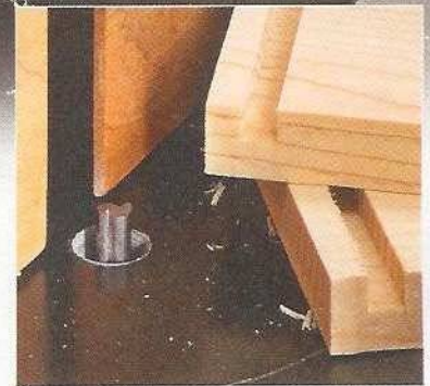
▲ One-Bit Drawers. Use a \frac{1}{4} " straight bit to rout flat-bottomed dados, rabbets, and grooves for this simple drawer joint.
