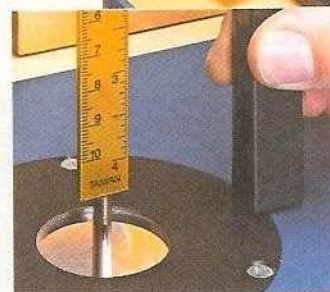
◀ Dual-Use. With the gauge standing upright, setting the height of a router bit is a snap.
