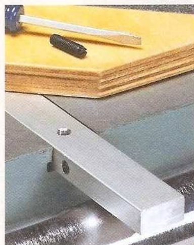
▲ Woodhaven . A small screwdriver is all that's needed to adjust the nylon set screws.
