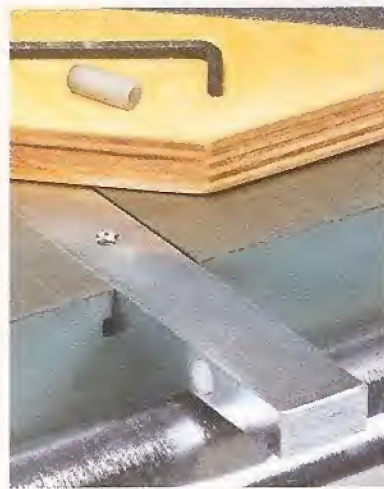
▲ Kreg. Use an Allen wrench to turn the nylon set screws in or out to fine-tune the fit in your miter slot.
