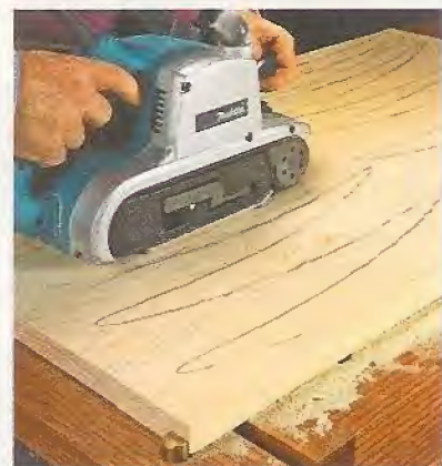
▲ With the Grain. Concentrate on one section at a time, and the crossgrain scratches will disappear quickly.
