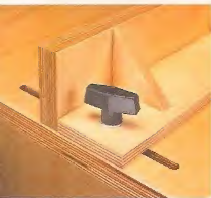
▲ Router Fence. Grooves in the router table allow you to easily position the fence and lock it securely to the tabletop.
