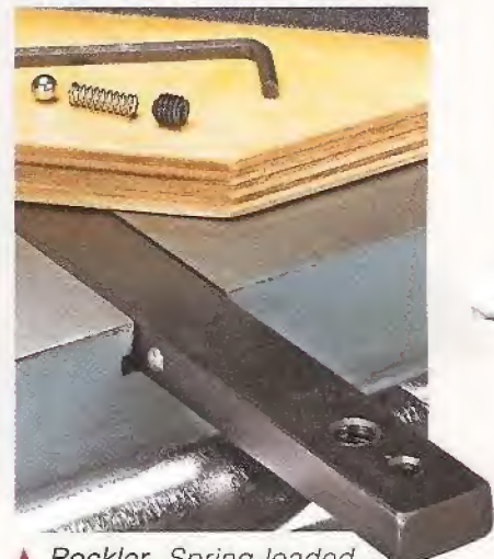
▲ Rockler. Spring-loaded ball plungers automatically adjust to fit the miter slot.
