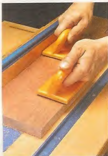
▲ Get a Grip. Besides keeping your fingers away from the bit, a pair of push blocks provide a grip on your workpiece that can't be beat.
