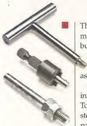
▲ Insert Tools. A purchased (top two tools) or shop-made installation tool (bottom) is the best way to get good results.
