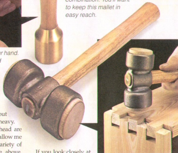
▲ Wood-faced Mallet. The cast brass head provides enough heft and the wood faces won't damage your work or tools.
