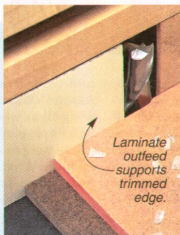
▲ Your Router as a Jointer. Use a carbide bit in your router table for smooth edges.
