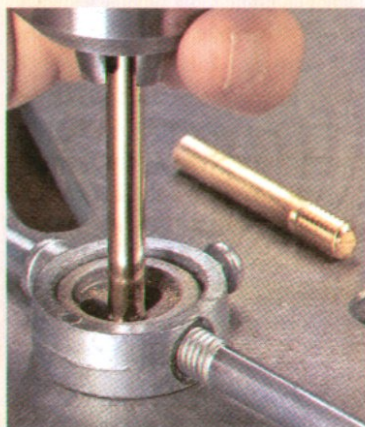
▲ Die-cutting the Rods. Secure the rod in the chuck and clamp the die cutter to the table. Rotate slowly by hand to cut the threads.
