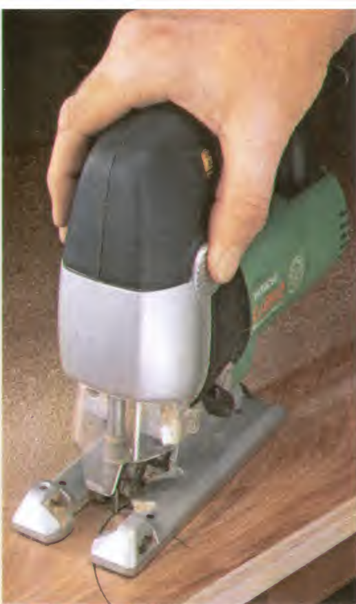
▲ Turn from the Front. Grip the saw directly above the blade when cutting curves. Take it slow, and let the blade do the work.
