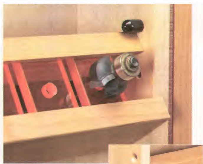
▲ Pivot Stop. Adding a pivot stop will keep the trays from pivoting too far. A vinyl cap will cover the screw threads.
