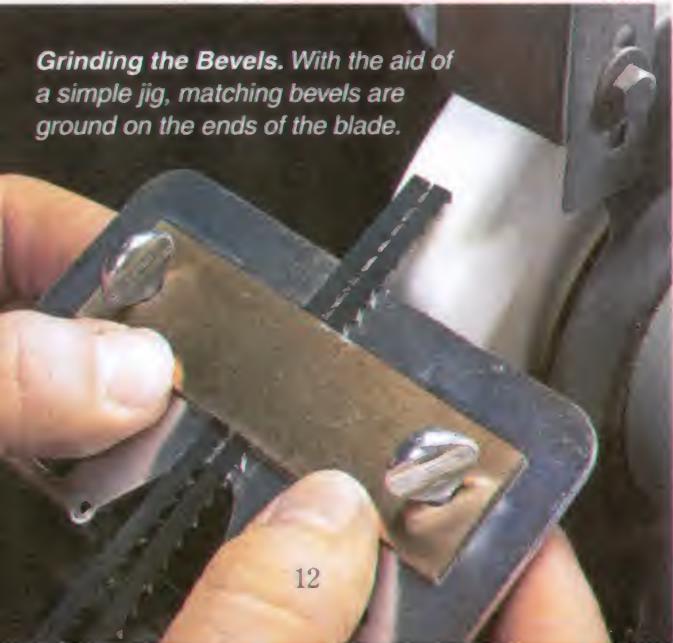
▲ Scarf Joint. To create a strong joint, the bevels should be at least a 1/8" wide to provide plenty of surface area for the solder.
