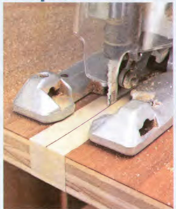
▲ Masking Tape. To help prevent tearout in the top face of the workpiece, you can apply masking tape to the cutline. The tape holds the fibers in place and keeps them from splintering.
