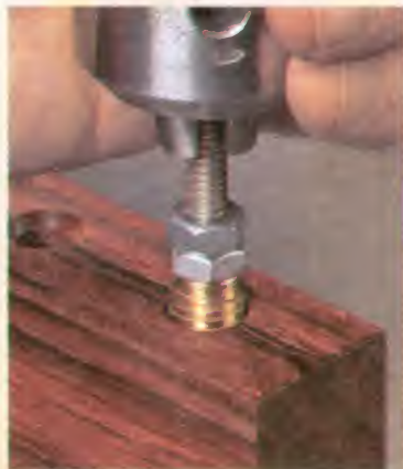
▲ Threaded Inserts. Using a piece of all-thread and two locked nuts, turn the chuck by hand to install the inserts.
