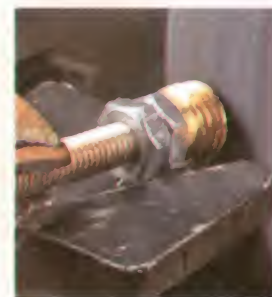
▲ Grinding Insert to Size. Use a long bolt and two nuts locked tight to secure the insert for grinding.
