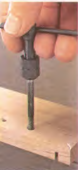
▲ Tapping the Holes. Cutting threads into the holes will hold the machine screws in place.
