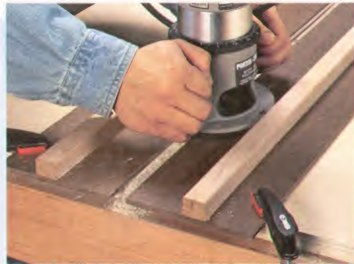
▲ Two Guides. Use two router guides to rout dados that exactly match your workpiece.
