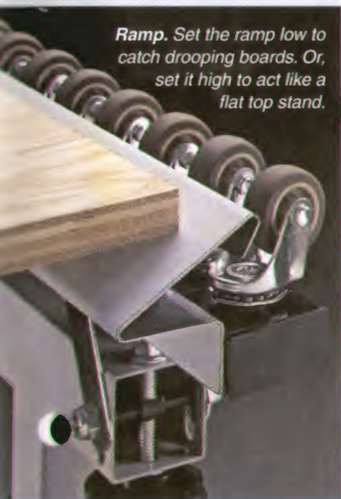
Swivel casters won't pull a workpiece away from the fence
