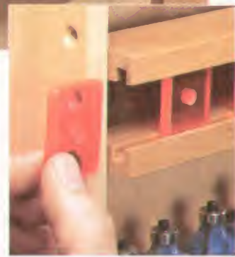
▲ Loading the Trays. Remove the pivot stop and turn the tray forward to add or remove bit holders.
