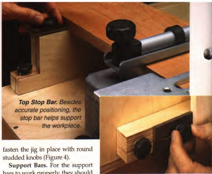
Adjustable Stops. These stops help keep longer workpieces square in the jig.
