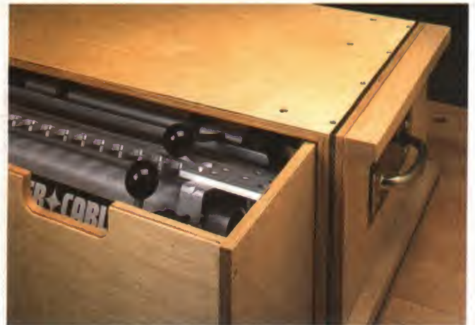
▲ Tucked Away. The large drawer is sized to hold the jig, templates, support bars, and knobs. And with the wings folded up, the workcenter stores neatly away.
