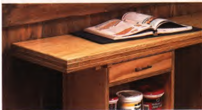
▲ Add a Worksurface. Put a little distance between the units and you can have even more worksurface just by placing a benchtop between them.
