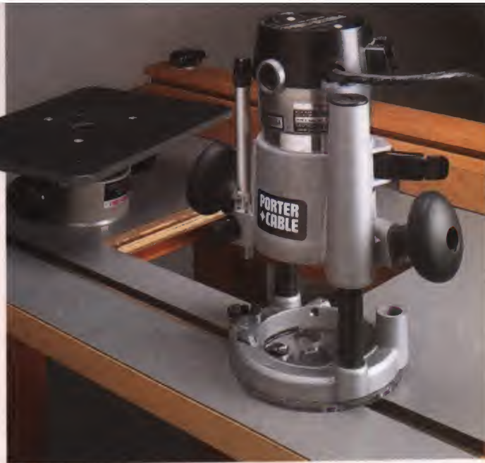
▲ Plunge Base. With an auxiliary plunge base, you can leave the standard base attached to your router table for fast changes between setups.
