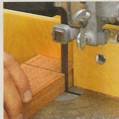
▲ Top/Bottom Shoulders. Use the same technique to make the remaining shoulder cuts.
