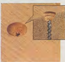
▲ Hidden Screw. Workpieces from old projects can have some hidden surprises beneath the surface.
