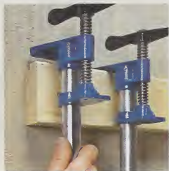
▲ Clamp Storage. To quickly store the Rockler clamp all you need to do is hang it by the built-in lip on the foot.
