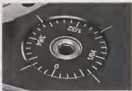
▲ The JessEm Rout-R-Lift. One full turn of the crank equals 0.05", with increments marked on the plate.
