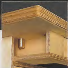
▲ Bench Dogs. A hidden pocket on each side of the top provides clearance space for bench dogs.
