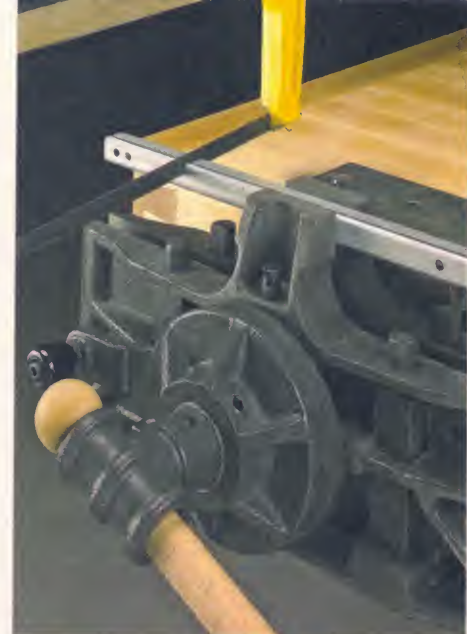
Verticality. Rotating the vise 90° provides a better grip on vertical workpieces.
