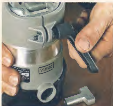
▲ In With the New. An inexpensive solution is to upgrade to an easy-to-grip, lever-type lock.
