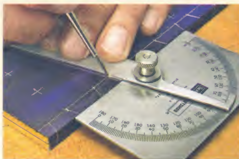
1 Use a protractor and scribe to lay out the tails on the brass sides. I used an angle of 15° for looks and strength.
