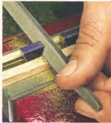
▲ Triangle File. For shaping tight corners and angles, different sizes of triangular files work great.
