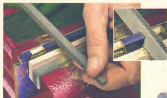
2 A square file quickly removes most of the waste. Then finish up the dovetails with triangular and needle files (inset).
