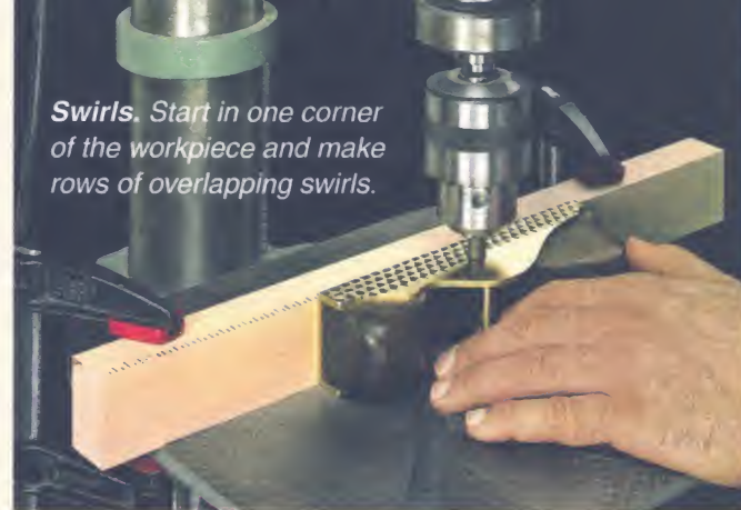
Spacing. Index marks laid out on top of the fence can be used to keep the spacing of the swirl pattern consistent.
