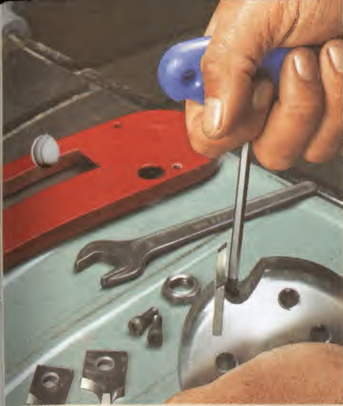
▲ Installing the Knives. Each knife is secured to the cutterhead with a sockethead set screw.
