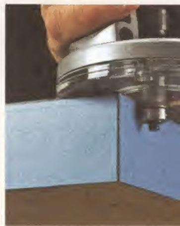
▲ Bearing Scratches. To prevent scoring of the laminate, check the bearing of the router bit frequently for glue buildup.
