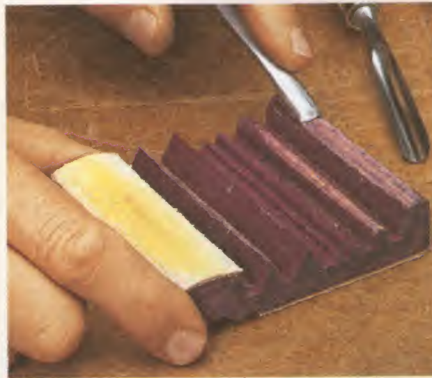
▲ Small Profiles. Paring chisels and carving knives can be made razor sharp on an inexpensive, profiled strop.
