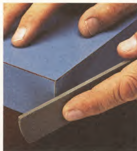
▲ Filing Edges. Downward and outward strokes of a flat mill file make smooth edges.
