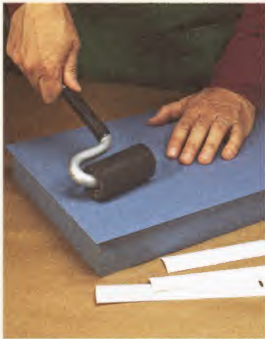
▲ J-Roller. Use a roller over the entire surface to apply pressure and eliminate air pockets.
