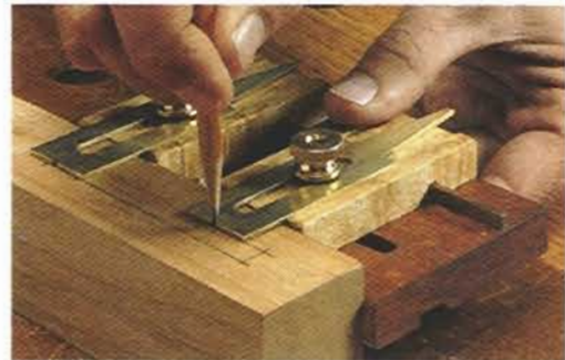
▲ Marking Mortises. First, use the tool to mark the ends of the mortise (top photo). Then set each key to a different depth to mark the sides of the mortise (bottom photo).
