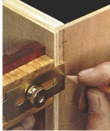
▲ Locating Screw Holes. Use the notch to hold the pencil tip while sliding the tool along the edge.
