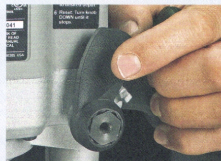
▲ Lever Lock. The most common type of plunge lock is a spring-action lever. You pull it back to release the lock.
