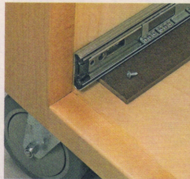
▲ Bottom Slide. A piece of \frac{1}{4} " hardboard positions the slide up off the bottom of the cabinet.
