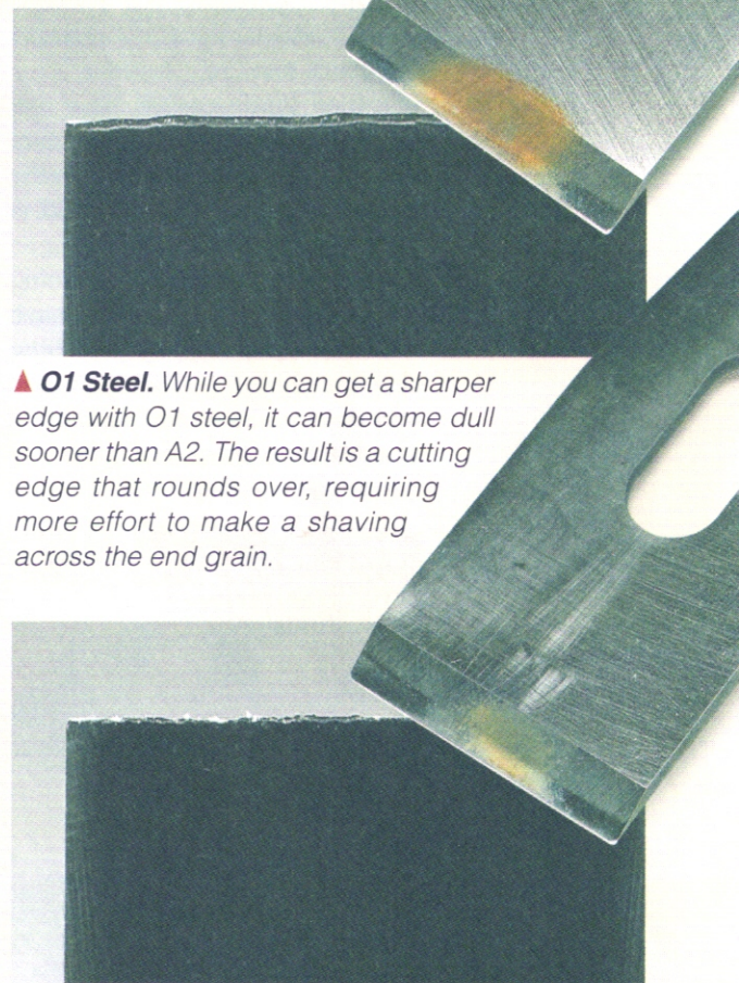
▲ A2 Steel. While A2 steel is harder than O1, the cutting edge is more fragile. It can break down, leaving a rough edge, but still be sharp enough to make a cut on end grain.
