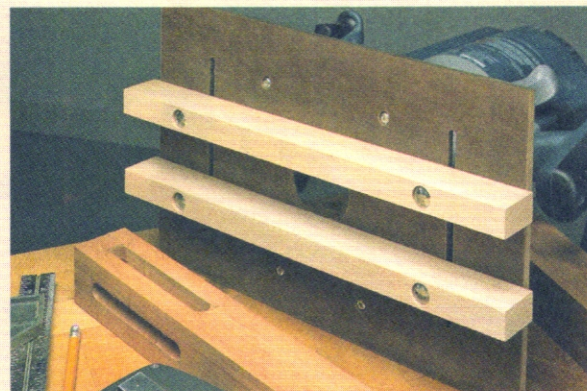
▲ A Simple Jig. The two adjustable guides sandwich the workpiece, giving you very easy and steady control of the router during the cuts.
