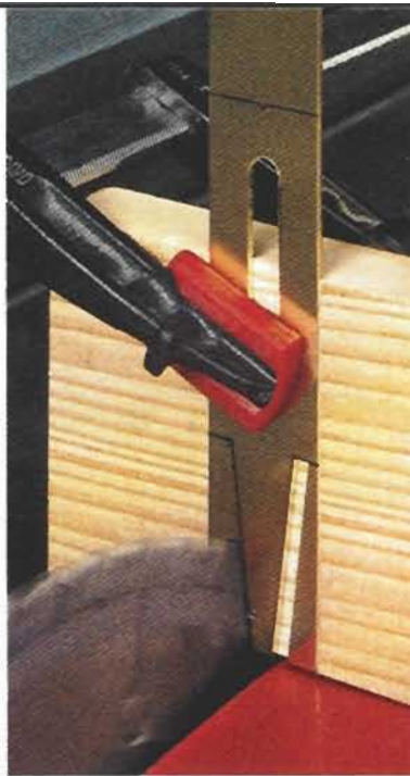
▲ Angled Cuts. Use an auxiliary fence with a shallow dado and clamp to hold the brass in place.
