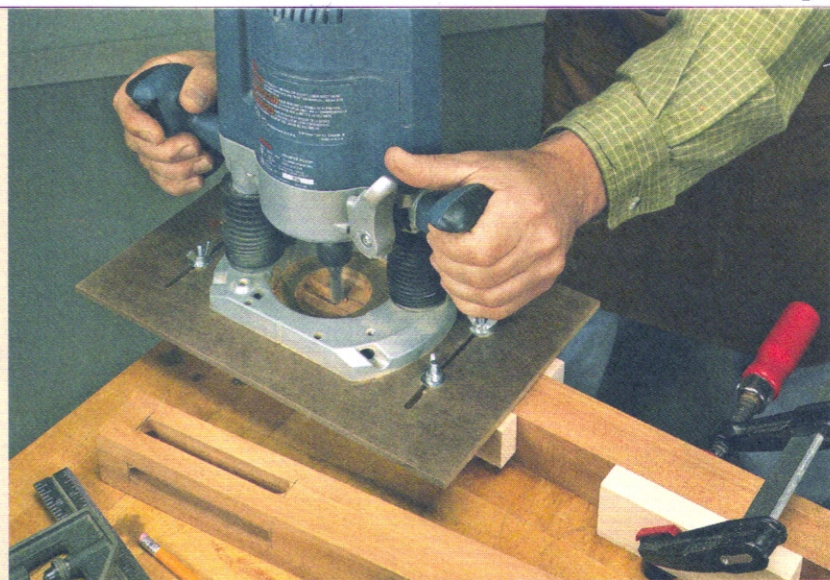
▲ Making the Cut. Once the jig is adjusted, routing the mortises is a simple operation. A stop block takes any guesswork out of ending the cut.
