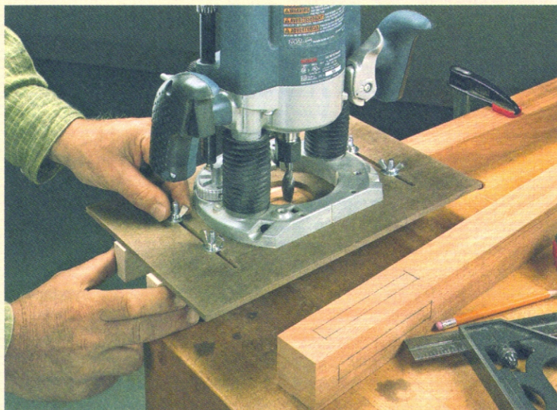
▲ Centering the Bit. Lower the bit to the surface and then reposition the jig to center it on the layout.
