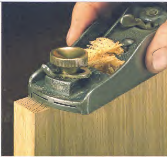
▲ A Tough Test. Shaving the end grain of a workpiece requires a keen cutting edge. As the edge dulls, the plane “chatters” and can’t make a clean shaving.
