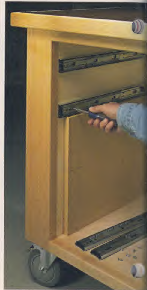
▲ Bottom Slide. A piece of \frac{1}{4} " hardboard positions the slide up off the bottom of the cabinet.
