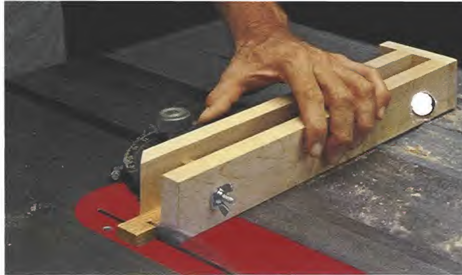
▲ Tight Between The Jaws. The jaws of the clamp can tightly grip even the smallest workpiece and keep your hands at a safe distance.
