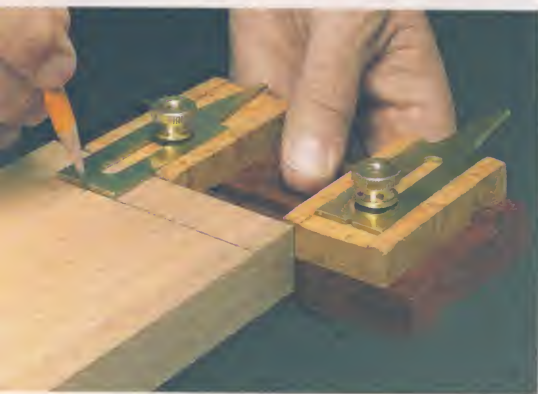
▲ Scribing Lines. A small notch in the end of each key holds your pencil tip for marking lines parallel to the edge of a workpiece.
