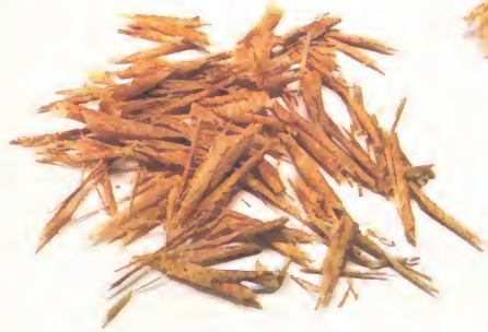
▲ A Tough Test. Shaving the end grain of a workpiece requires a keen cutting edge. As the edge dulls, the plane “chatters” and can’t make a clean shaving.
