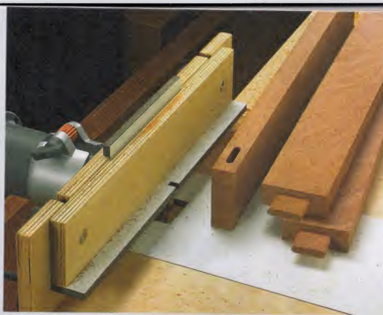
◀ Perfect Mortises. An ordinary straight bit and a simple hold-down is all it takes to rout mortises using the multi-tool.
