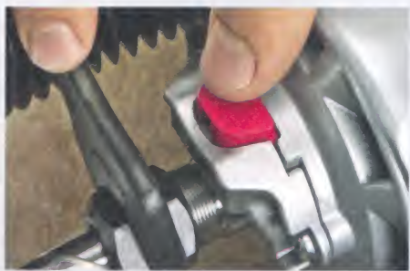
▲ Spindle Lock. Depressing the button locks the spindle so the collet can be tightened or loosened with one wrench.
