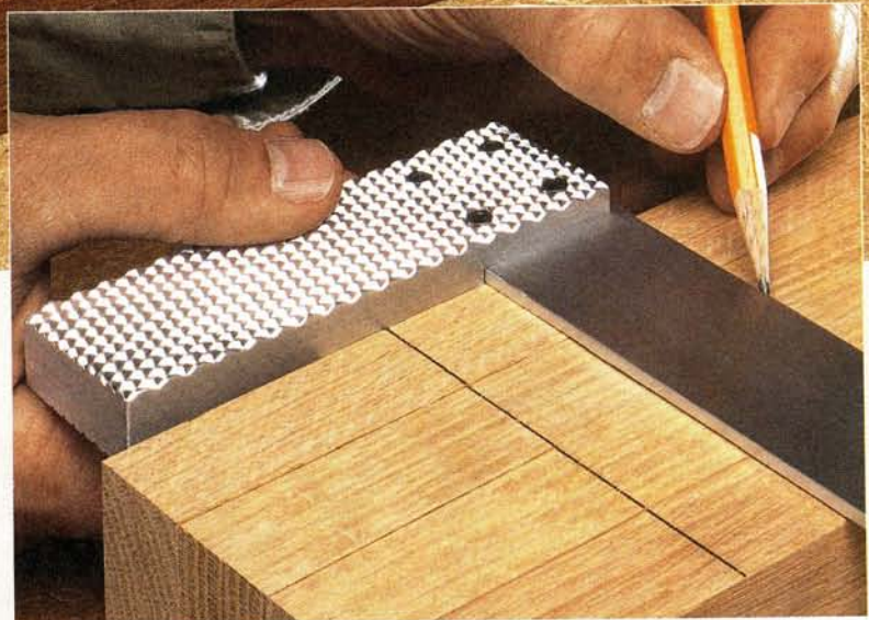
▲ Diamond Pattern. With a simple sled for your table saw, you can create this attractive diamond pattern. For details, refer to page 17.
