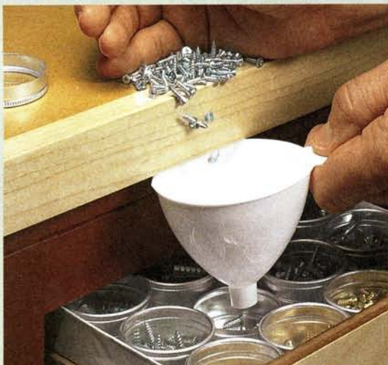
▲ Ellis Biderson of Huntington Beach, CA, uses a funnel to help manage small parts after he is done using them. He simply positions the funnel over an open container and then scoops the parts into the funnel to return them to storage.
