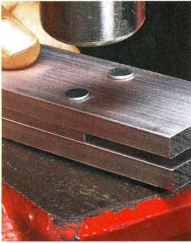
▲ Riveting. A few taps with a ball peen hammer will “mushroom” the ends of the rivets for a tight fit.
