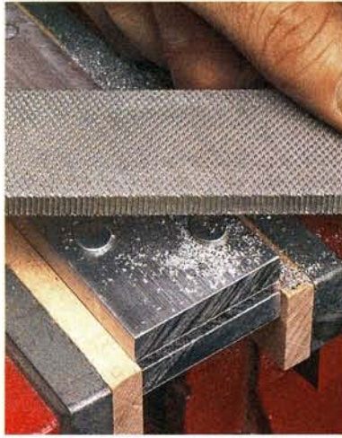
▲ Filing. A file makes quick work of smoothing the rivets flush with the surface of the workpiece.
