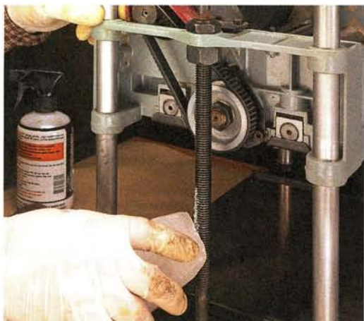
▲ Protection. Paraffin wax on the posts and spindles of the cutterhead provides protection and allows for smooth movement.
