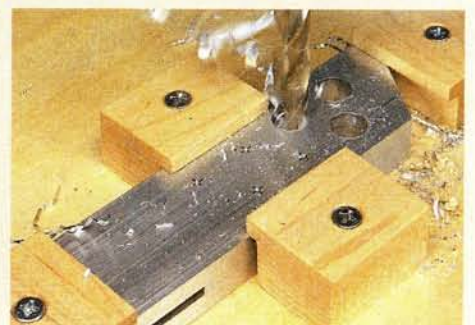
▲ Hole Pattern. Use a \frac{7}{16} "-dia. bit to drill the decorative hole pattern on the handle. A countersink forms the \frac{1}{16} " chamfer around the edge of each hole.
