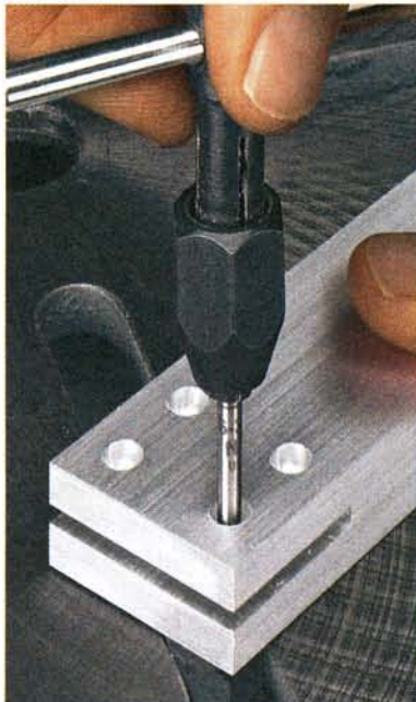
▲ Tapping Threads. Cutting threads in soft aluminum is a snap with a hand tap and lubricant.
