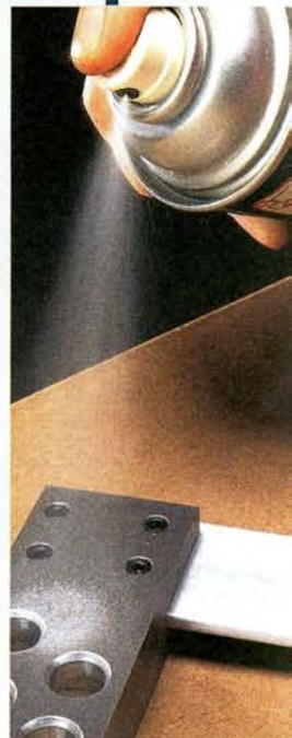
▲ Wax. A couple coats of paste wax adds a nice gloss and keeps the aluminum from staining your hands black.
