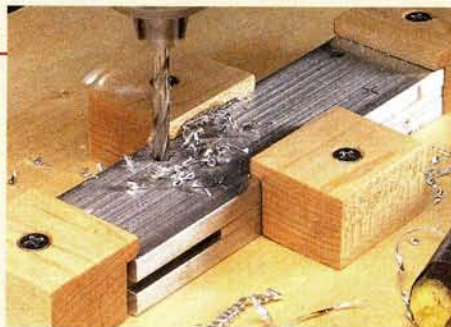
▲ Rivet Holes. Drill \frac{1}{4} "-dia. holes for the rivets, then check the fit. The rivets should slip easily into the hole and completely through to the other side of the blank.
