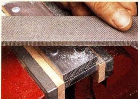
▲ File Flush. A coarse file makes quick work of removing the excess material from the rivets. File just until the rivets are flush. You'll sand them smooth later.
