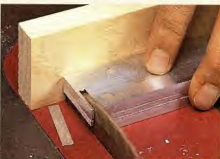
▲ Trim Edges. Use a carbide-tipped blade to trim the blank to final length and square up the sides. Then trim the corner off the end as shown in Figure 2.
