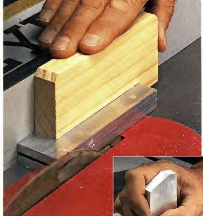
▲ Trimming Edges. A notched push block makes it safe to trim aluminum with a carbide blade.
