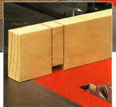
▲ Notch It. A notch in an auxiliary miter gauge fence pinpoints the dado location on the workpiece.
