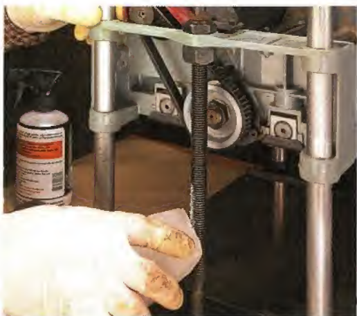
▲ Protection. Paraffin wax on the posts and spindles of the cutterhead provides protection and allows for smooth movement.
