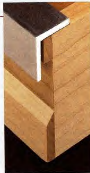
▲ Low-Profile Pull. A length of aluminum angle makes an easy-to-grip, low-profile drawer pull.
