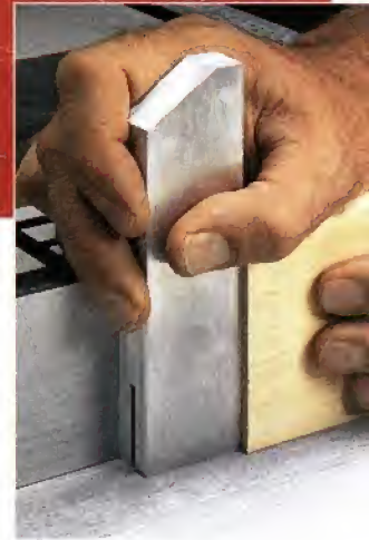
▲ Trimming Edges. A notched push block makes it safe to trim aluminum with a carbide blade.
