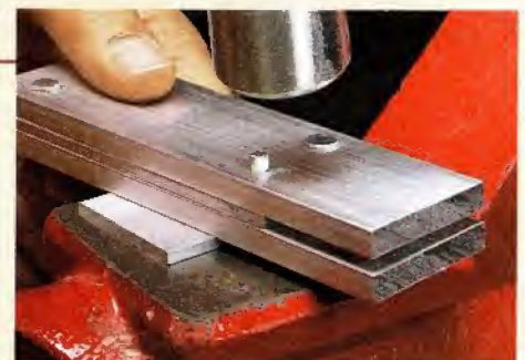
▲ Adding Rivets. A spacer raises the handle so you can "mushroom" the ends of the rivets. Remove the spacer and flip the blank over topeen the other side.
