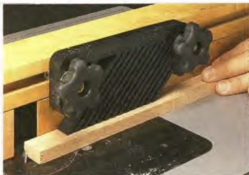
▲ Fence Mount. A fence-mounted featherboard ( Rockler ) improves the cut by providing downward pressure on a workpiece.
