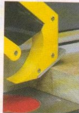
▲ Ramp. A piece of aluminum provides a smooth, durable surface to guide the hood over a workpiece.
