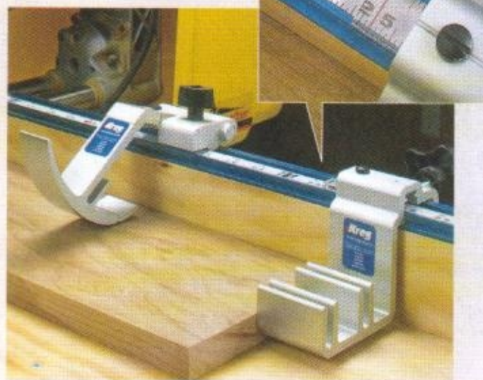
▲ A Pair of Stops. Both the flip-stop (left) and the fixed stop (right) feature an easy-to-read hairline cursor (inset above) for making accurate cuts.
