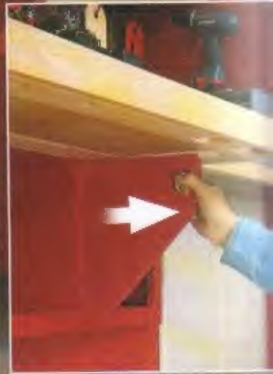
► Sliding Supports. Sturdy bench brackets slide out to level the workbench and make for a stable worksurface.
