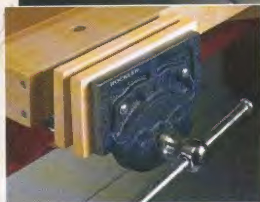
◀ Face Vise. A simple, bolt-on face vise is a handy addition to any bench. Wood jaws protect the workpiece.
