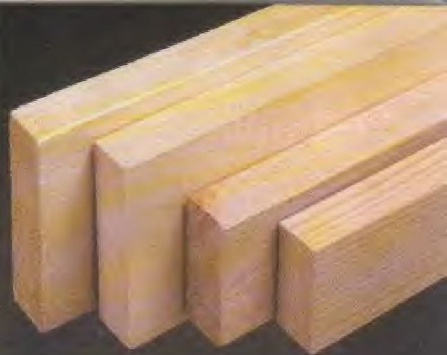
Jointed and Planed. Your stock will end up a little narrower and thinner after flattening and squaring, so plan for the reduced dimensions.
